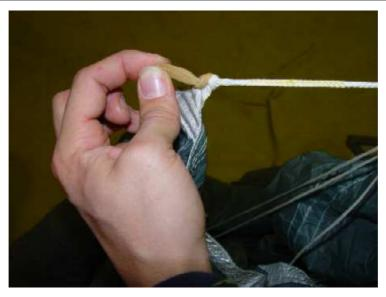
The next step is to check if the stabilizers and their slider stops are in the proper position outside the suspension lines. If the stabilizer (or its slider stop) lies under the line, the canopy could possibly become damaged. The canopy stowed in this way should look like in the picture.
