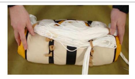
After the suspension lines are put into rubber sleeves on the main canopy deployment bag, fold the remaining suspension lines with harness risers and prepare the parachute container for the storage of the bag with suspension lines and harness risers.
