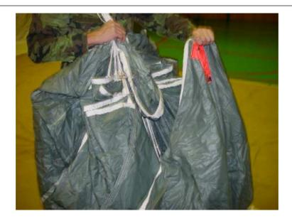
Roll the canopy trailing edge evenly around the stowed canopy and align the left and right sides in such a manner that the seams and trailing edge trims are placed against each other.
