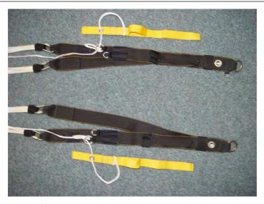
The auxiliary control loops are placed nearer the centre. The placement and connection is shown in the picture.
