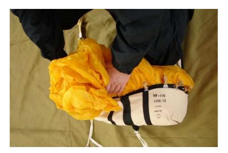
After the main canopy is stowed into the bag, smooth it inside. Pay attention to the canopy trailing edge central seam and the warning label that must be placed symmetrically in the centre. The even placement influences a symmetrical canopy opening.
