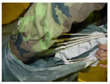
As you have pulled out the canopy between the line groups A and B, do now the same between the lines C and D. Pull out the fabric fold between both groups outside to both sides. If you look down among the stabilizer folds, the flaked folds should look aligned as shown in the
