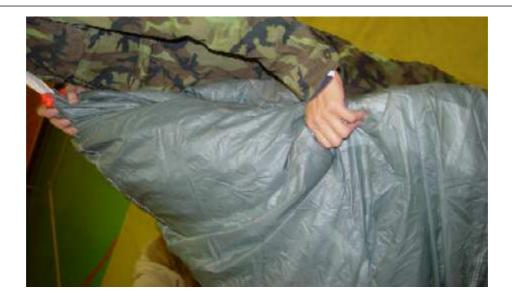
Insert the rolled-up trailing edge part into the parachute centre (see the picture).
