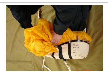
Start pulling the container over the canopy, first one side, then the other one. Keep the stowed canopy corner on top during the container pulling-over, then roll up the canopy into the container corner. If so, it will be easier to press the canopy into corners and the packed canopy will look neater. Only when the whole canopy is placed inside the container, release the pressure of your knees. The above described procedure helps to fully fill the container corners and keeps the centre pressed.
