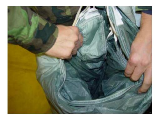
Due to a lot of fabric between A and B line attachment points, it is easy to differentiate both line groups: look down inside the small S-shaped fold on the stabilizer and find "excess" fabric.
