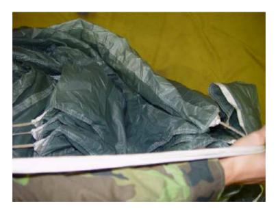
Fold the trailing edge into S-folds in a similar way such as stabilizers. Stretch the steering lines and auxiliary steering lines and turn the excess auxiliary steering lines twice around the forefinger and middle finger of the left or right hands, and put the resulting twist into a rubber sleeve placed on the fourth steering loop in the direction from the parachute beginning to the parachute centre.
