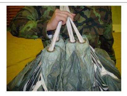
"Flake" single cells of the parachute leading edge. "Flake" the whole leading edge with one hand as shown in the picture – and begin from the end cell chamber that is nearest your legs. Stretch out each cell chamber and hold in your hands. After you stretch another one, put this cell chamber to the previous one, be careful so that you will not let any pulled out cell chambers slip before you hold fast all the cells in your hand.
