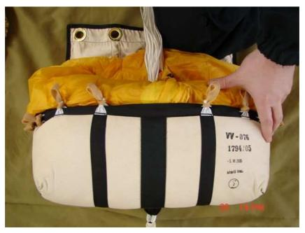
Close the deployment bag with a suspension line bundle. Put the remaining suspension line length into rubber sleeves so that the length of single loop is between 5 and 7 cm.
