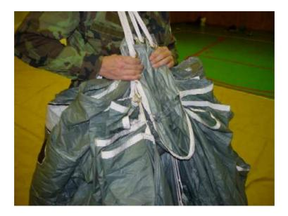
Now touch down and hold the trailing edge exactly in the centre, there is an sewn-in identification mark to find it easier.
