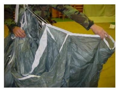
Pull out and fold side stabilizers on each side. Set the centre (by moving your hand downwards between the two front rings – exactly one half of all the lines will be on one side, the other half will be on the other side). Let the middle cell hang and at the same time divide all the remaining cells on one side to the left and right sides.
