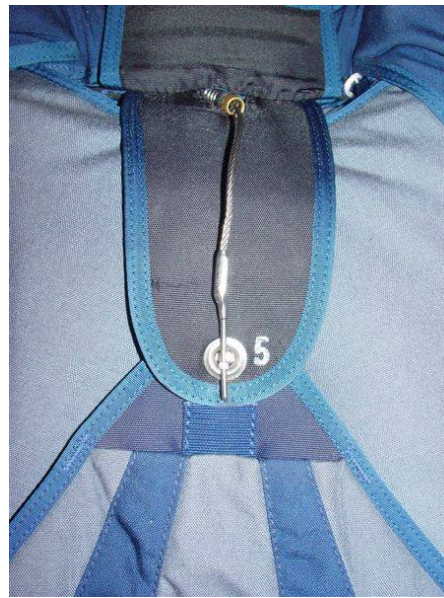
New way of packing. The sequence of the reserve parachute flaps packing 1-2-3-4- 6-5 .
