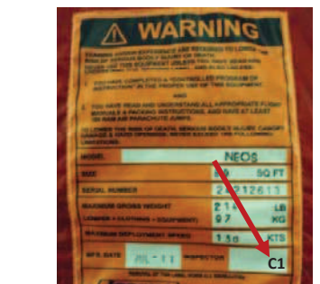
Fig. 17. When the modification is completed, mark "C1" with permanent marker in the inspector box on the warning label.
