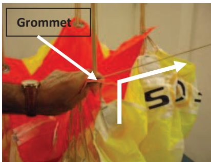
Fig. 12. Pass the C1 line through the corresponding slider grommet.
