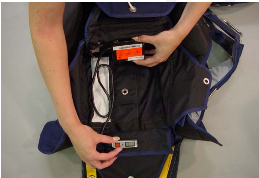
Cypress AAD prior to installation.
