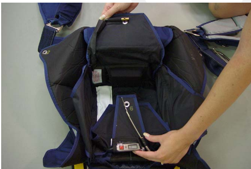
Cypress AAD after installation.
