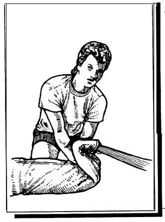
**35.** Move to the **side** of the canopy and put one hand **under** the slider edge of the **bundle**. **Place** the other hand on top a **little** farther up.
