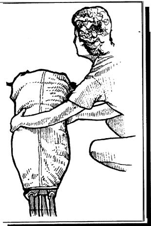
**34.** Tuck the sides under, starting at the slider and working up, making the canopy into a flattened cylinder shape.
