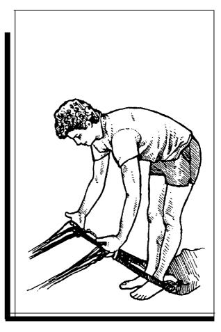
2. Stand between the right- and left-hand riser groups and start moving up the lines, allowing them to slide between your fingers. Push the slider ahead, until you reach the lower surface of the canopy.
