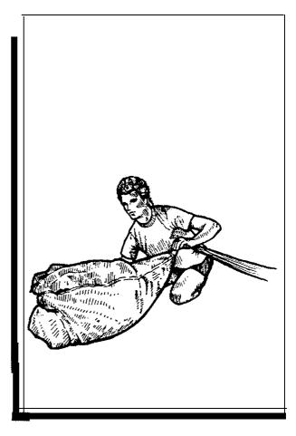
**33.** As it rests on the floor, the canopy should be triangular in shape as shown.
