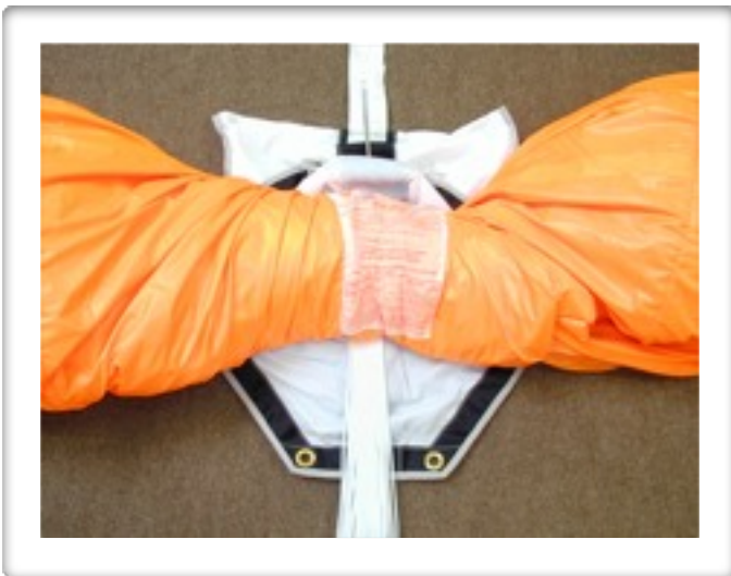
Lift up the base gently and pull the free bag underneath it. By using a T Bodkin you can make sure the base sits right at the spot where the loop will pass through later on.
