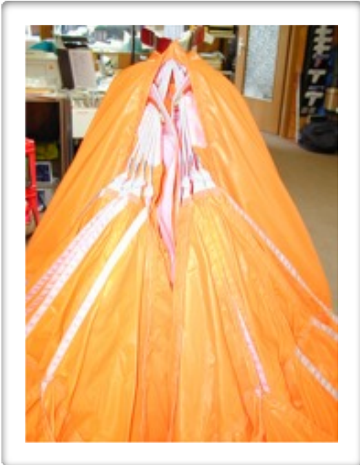
Close up shot of a properly dressed nose, with the slider in the centre and the trailing edge behind the flaked nose
