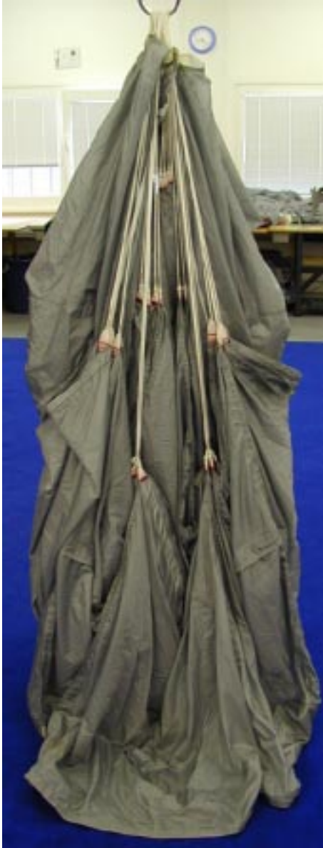
Correctly folded canopy shown from trailing edge side
