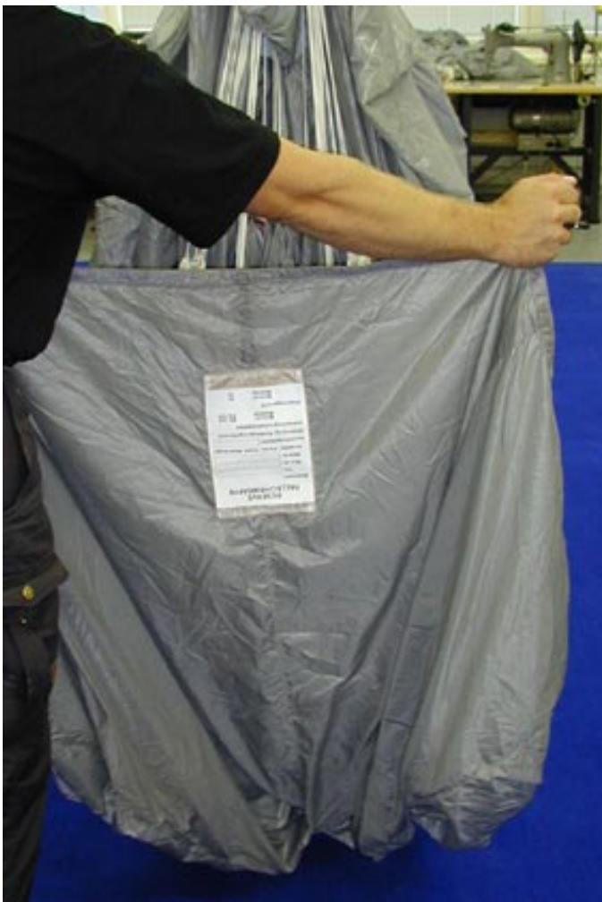
Step 8 Pull up the centre cell with the trailing edge and position it just above the slider grommets and around the line strand See details on next page.
