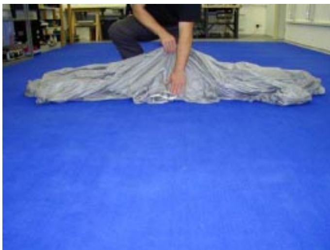
Step 15 Dressing the centre cell in it's reefed configuration
