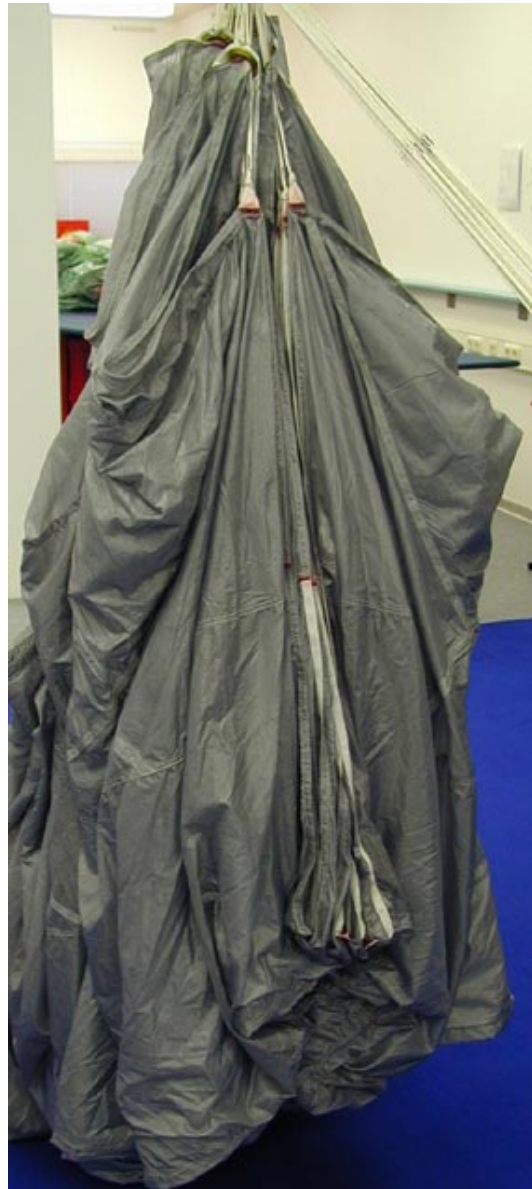
Correctly folded canopy shown from leading edge side
