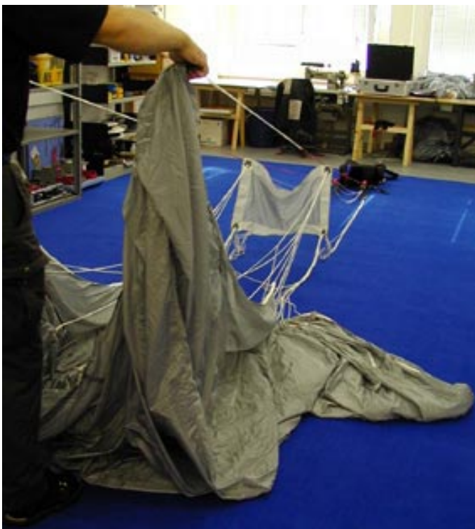
Step 2 Perform a line check by making sure the steering lines run free through the slider grommets to the steering toggles
