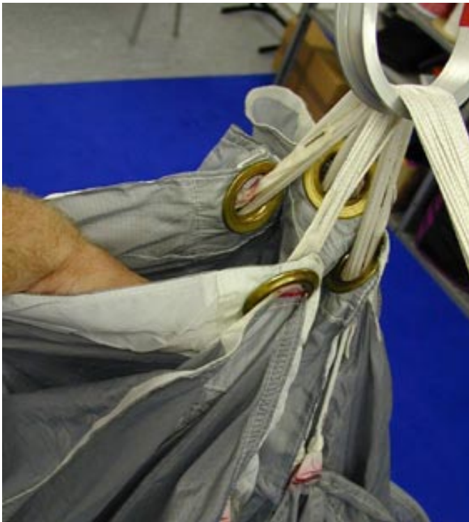
Step 7 Position the slider in the centre of the canopy
