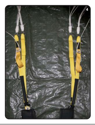
Set the deployment brakes according to the manufacturers instruction of your harness container system or riser manufacturer.
