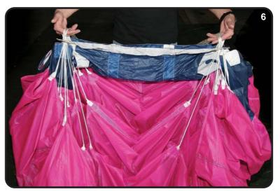
The tail should be farthest from the rig and the nose openings should be facing the rig. If the reverse is true and the rig is positioned correctly as described earlier, then the parachute was attached to the harness backwards! If you do not know how to solve this problem, get qualified assistance from a FAA rated rigger / instructor or a proper rated equivalent of your country.
