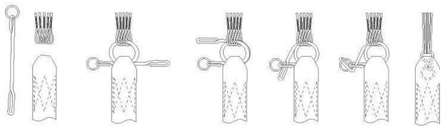
Secure the Soft Link ring in the webbing pocket, and hand tack as shown.
