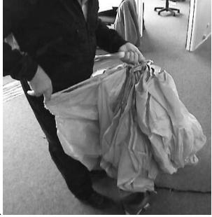
Holding the cell inlets firmly, shake the canopy vigorously to clear the fabric from the lines. Then, on one side of the canopy, separate line groups A & B and fold.
