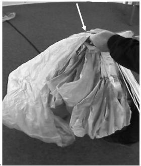
Clear each side of the tail and bring them around towards the front (nose) of the canopy. It is very important to make sure that no (steering) lines pass in front of the leading edge (nose), as this may cause a line-over malfunction.
