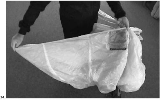
Join the two air inlets in front of the air inlets (the leading edge) and roll the tail between the two arrows, making sure not to catch the leading edge in to the roll. Never lose the grip on the line bundle and the slider.
