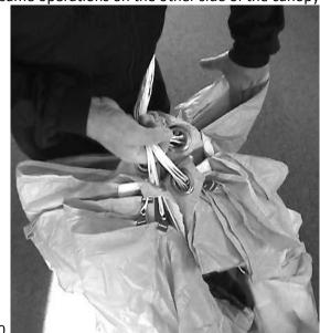
This is a view of the flaked canopy. While keeping the nose pointing towards yourself, check that the slider is properly spread out between the 4 line bundles (front, back, and right, left) and that the slider grommets are pushed up against the slider stops. Note that all (steering) line attachments are at the center.
