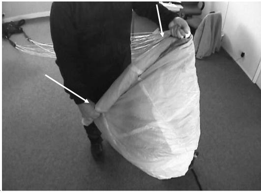
Gently swing the canopy out and lay it on the floor as shown. Carefully push the air out of the canopy. Again, make sure that the slider stays in place against the slider stops. WARNING: IF THE SLIDER IS NOT AGAINST THE SLIDER STOPS, THE POSSIBILITY OF A HARD OPENING AND SERIOUS INJURY OR DEATH IS SIGNIFICANTLY INCREASED.
