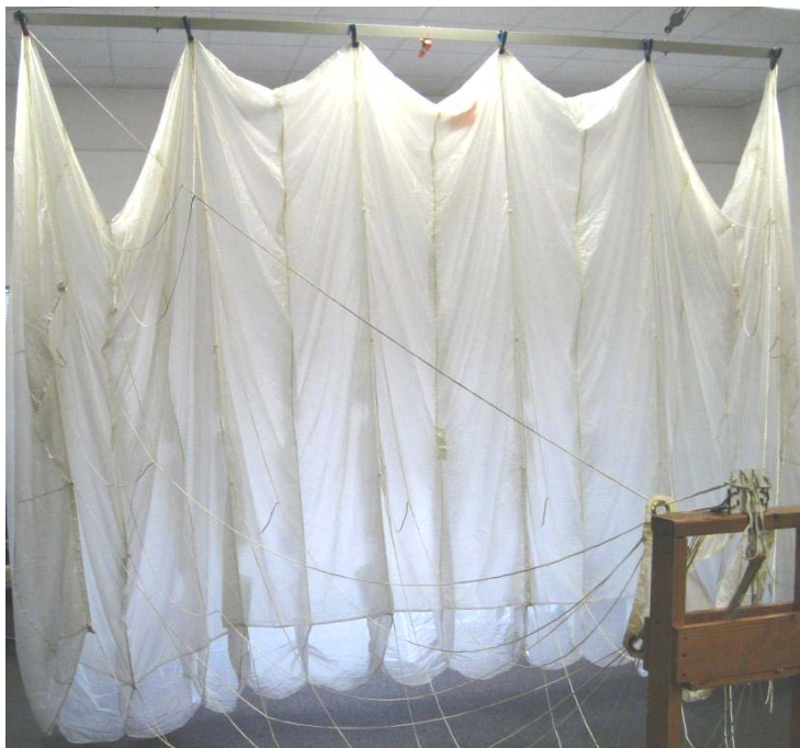
Hanging the canopy by the tail helps in both assembling and inspection.
