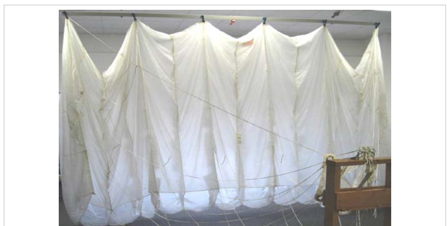
Hanging the canopy by the tail helps in both assembling and inspection.
