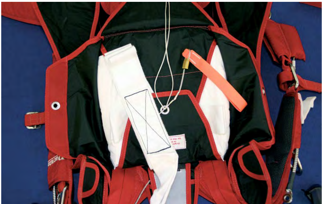
Picture 5 Close flap # 2 and S-fold the rest of the bridle to one side. (Should give you circa 6 folds)
