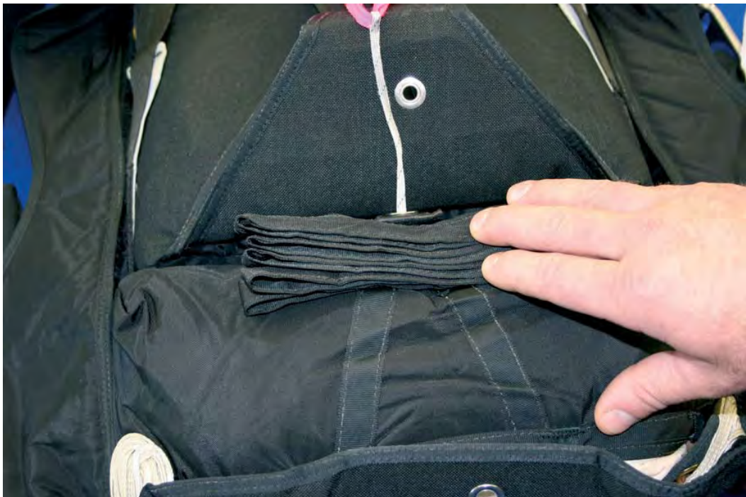
Picture 40 Fold the main bridle in S-folds under the loop keeper on top of your bag.
