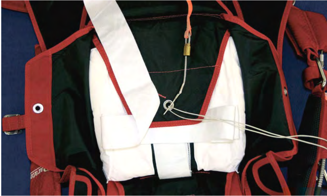
Picture 4 Stow the first section of bridle under flap # 1 using 2 complete S-folds, pinching them under flap one, just before the grommet, yet preparing the rest of the bridle to be folded up in S-folds as shown in the picture above.
