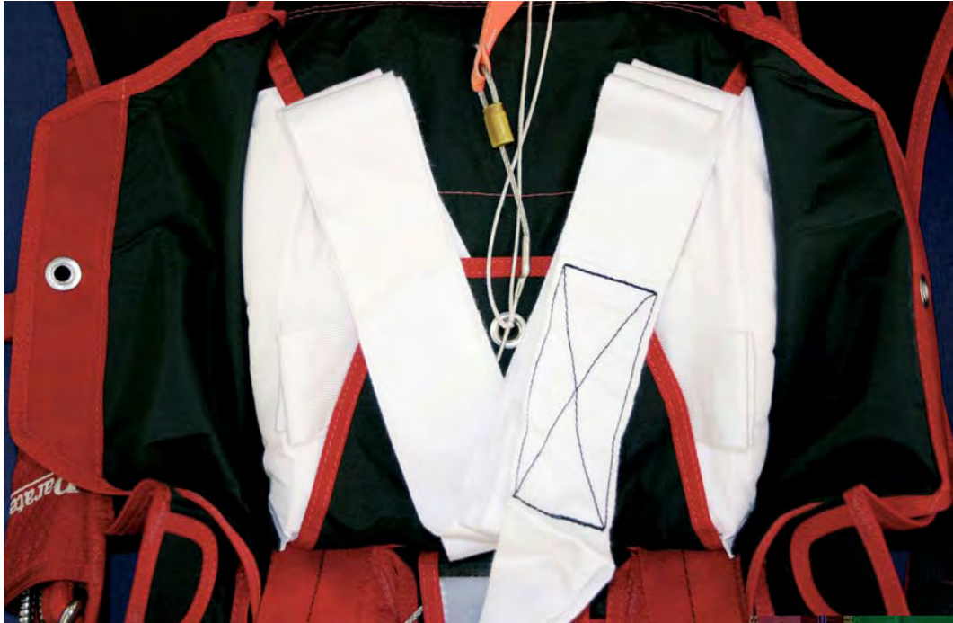
Picture 6 Count half of your folds and move them together to the other side, creating a V of S-folds this way.
