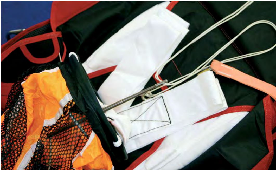
Picture 7 Place the bottom rim of the spring pilot chute on the base of the V, to keep it in place. Using a gun cleaning rod or similar device with an eyelet on the end to pull the cord through makes things quite easy, assuring that your pack job doesn't shift.
