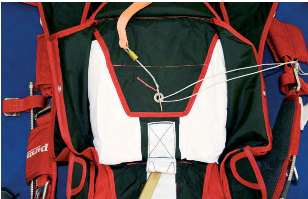
Picture 3 Close flap #1 and stow the x box stitch connection to the bridle under the free bag.
