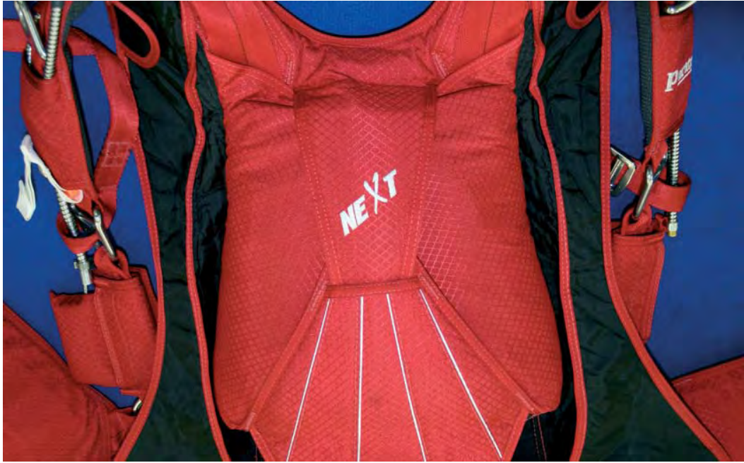
Picture 16 Seal, and document your pack job. Close the pin cover flap by using the side tuck tabs. The NEXT is now ready to be assembled with a main parachute.
