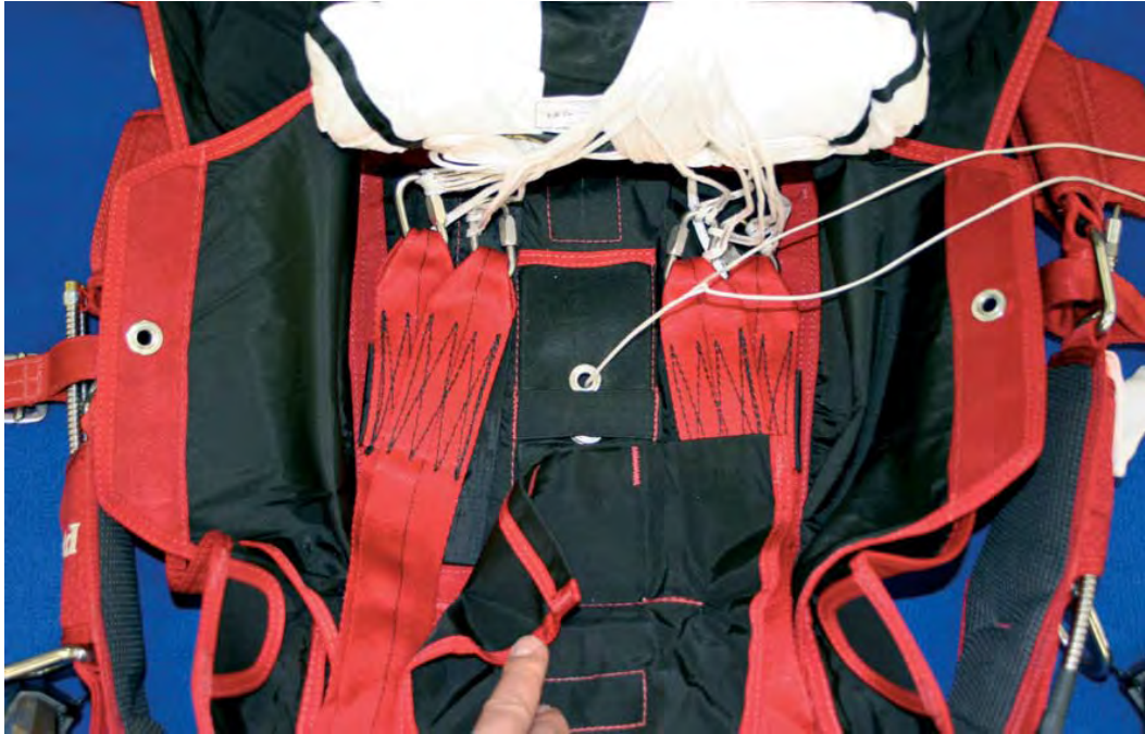
Picture 2 Please make sure that the reserve risers are being placed UNDER the covers of reserve flap # 2.
