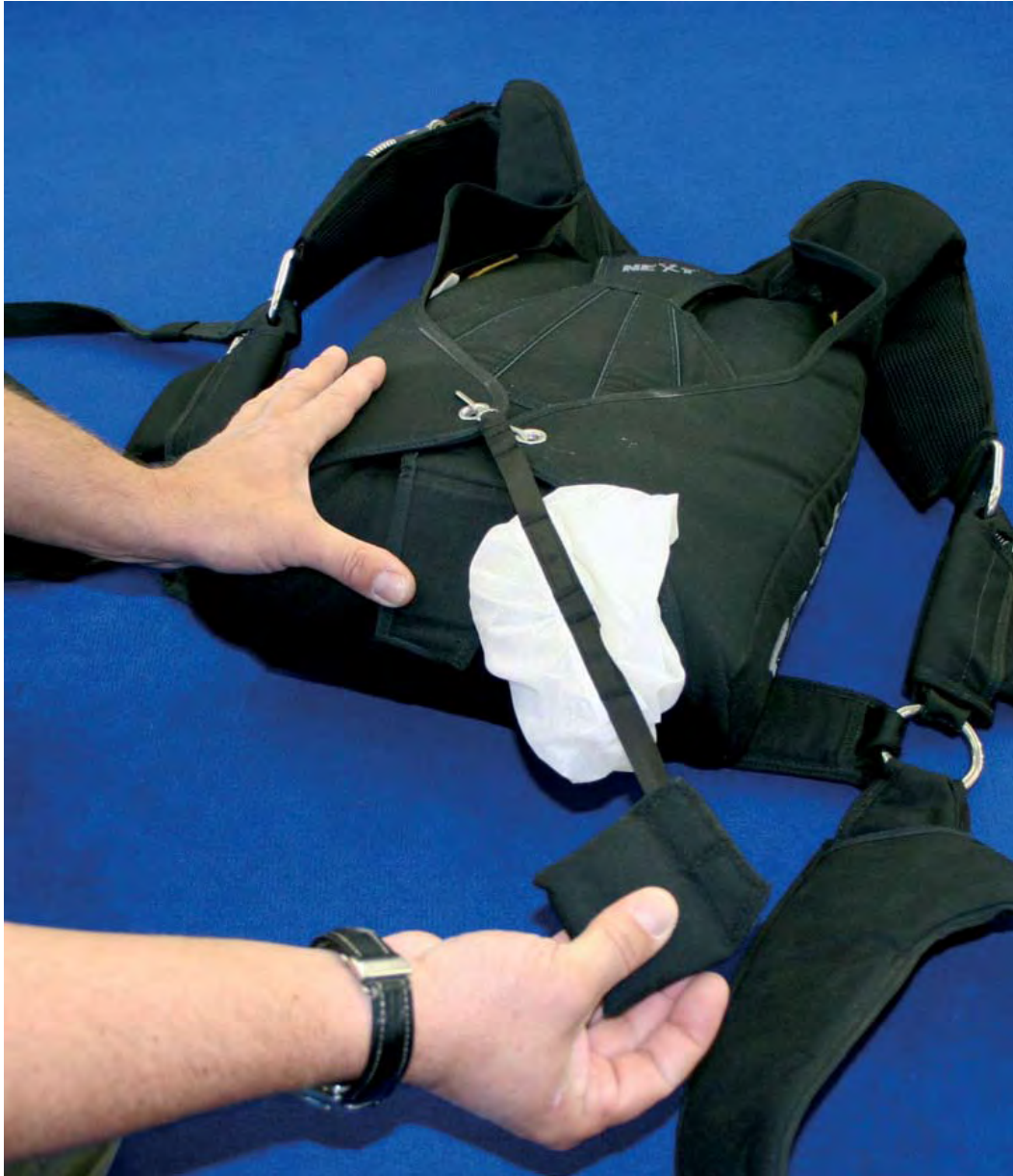
Picture 45 Close the left side flap, secure the closing pin and close the pin cover flap.
