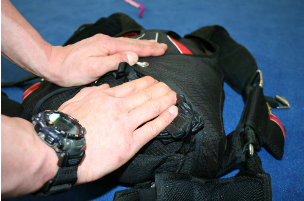
Picture 46 Push the access fabric of your pilot chute under the right side flap.
