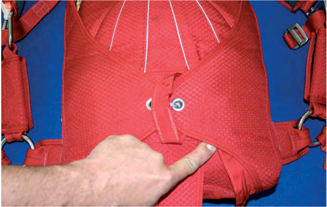
Picture 26 Stow the excess bridle under the bottom of the right side flap.
