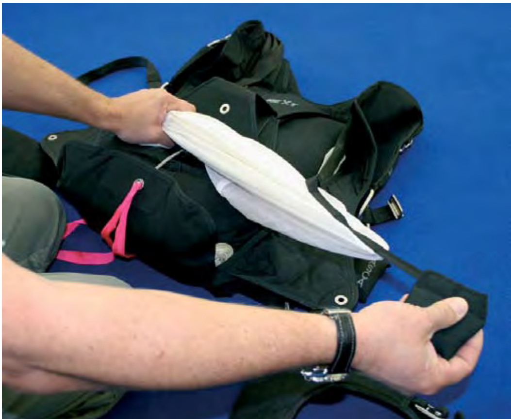
Picture 42 This is a very important step: Hold the pad with your right hand and straighten out the pilot chute, by moving with your left hand down to the opposite end holding the pad
