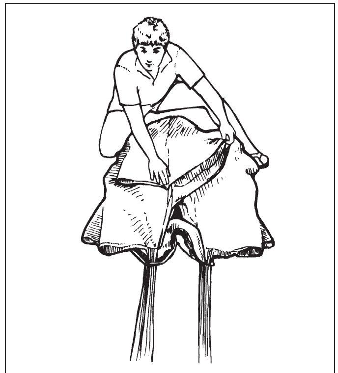
I. Return the center tail tab to the bottom center of the bundle. Where the stabilizers attach to the main body of the canopy. “Cocoon” the canopy to the width of the bag.
