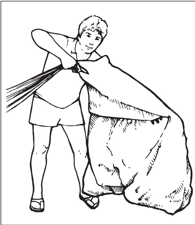
F. Kneel at the top of the canopy facing the container. Draw the canopy toward you while at the same time narrowing the bundle to the width of the bag. Constantly work the fabric away from the links.
