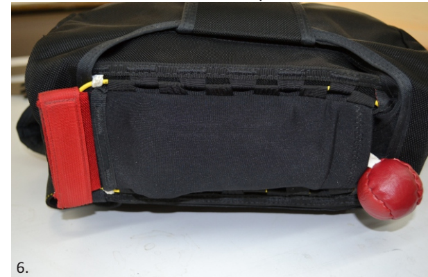
Stow Main Pilot chute in BOC pouch
