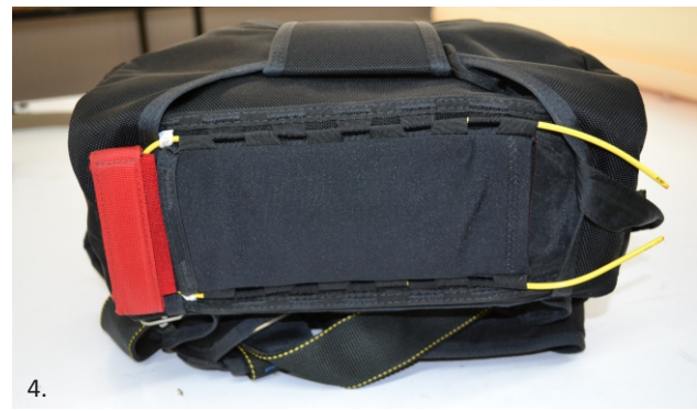
Stow Main Pilot chute in BOC pouch
