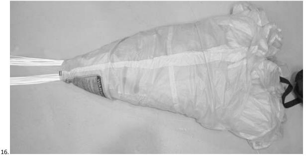
S-fold the canopy bundle as required for the D-bag. Then gently slide the canopy into the D-bag.
