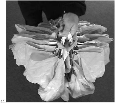
Pick up the center cell by its leading edge (identified by small red tape) and lay it on top of the lines just below the slider. Hold firmly, and make sure that the slider stays in place, pushed up against the slider stops. Also make sure that the steering lines remain in the center and at the back.
