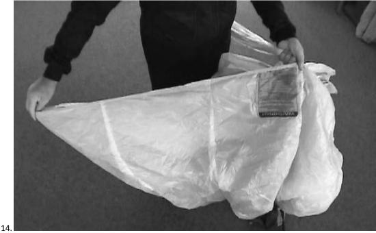
Join the two air inlets in front of the air inlets (the leading edge) and roll the tail between the two arrows, making sure not to catch the leading edge in to the roll. Never lose the grip on the line bundle and the slider.
