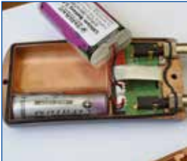
IV. Remove the battery from its location and unplug Battery Pack.
