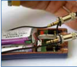
IV. Lift PCB and disconnect the two connectors.
