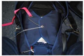
11. Close the bottom flap #5 (picture 11a). Close top flap #6 (picture 11b) and insert the reserve pin through the eye of the reserve cable first, then through reserve closing loop. Make sure to tuck the closing pin under the protector pocket.
