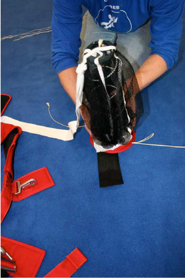
Place pilot chute upside down onto the compression strap
