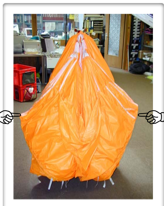
Extend the flakes of your nose left and right to fully cover the trailing edge
