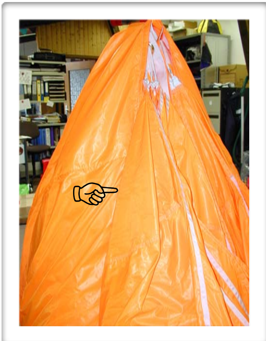
Bring up the tail Position the trailing edge of the centre cell on the lines and bring the corresponding sides of the trailing edge around the canopy, placing them BEHIND the outermost cells
