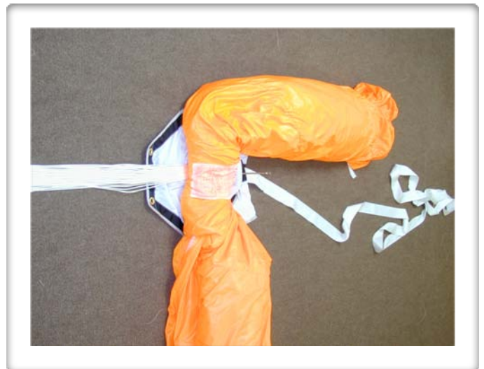
Bring the first „ear“ forward to sit at a 90° angle from the base
