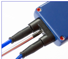
I. Unscrew Connectors Locking Clip (CLC)
