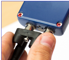
II. Remove Connectors Locking Clip (CLC)
