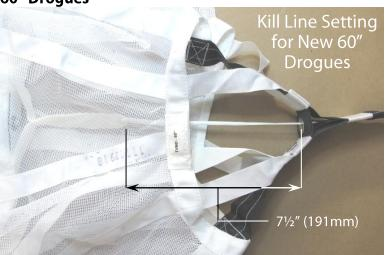
Using the same technique as above applying about 10 lbs. of tension, the larks head knot at the bottom of the kill line attachment bridle should be 7½" (191mm) above the kill line guide grommet on New Drogues (factory setting).
