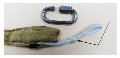
Drogue collapse is calibrated for average weight and fall rates, if you feel the drogue is collapsing too far with longer than normal "trap door" you may lengthen it a little bit by untying the knot and letting out required length of finger trap. Ideal trap door time is 34 sec. with a minimum of ½ sec.
