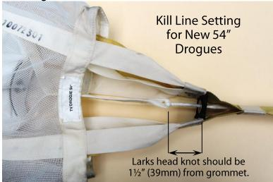
Apply about 10 lbs. of tension against the Kevlar bridle and with the other hand apply the same tension on the kill line by pulling on the kill line attachment bridle or the drogue handle. The larks head knot at the bottom of the kill line attachment bridle should be 1½" (39mm) above the kill line guide grommet on New Drogues (factory setting).
