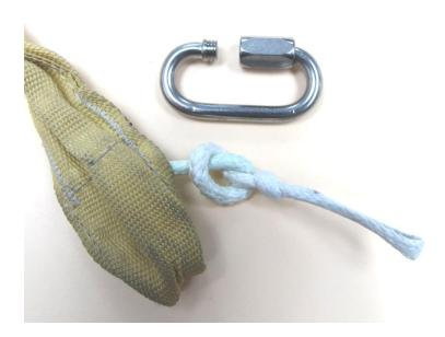
If you notice a kill line that is too long, a simple overhand knot, tied within the finger-locked section of the kill line, at the deployment bagend, will effectively shorten it almost 2" (51mm), and bring your drogue collapse system back into trim.
