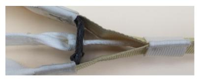
If this distance is more than 1" (26mm) less, the larks head knot will impact the guide grommet at high speed, quickly causing damage to both. However, in this instance, deployment, while slightly slower, will still happen more or less normally.
