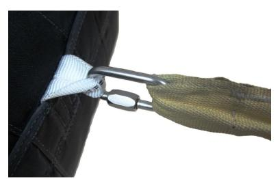
To check this relationship: Anchor the rapid link at the deployment bag end of the drogue bridle.
