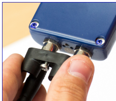
II. Remove Connectors Locking Clip (CLC)
