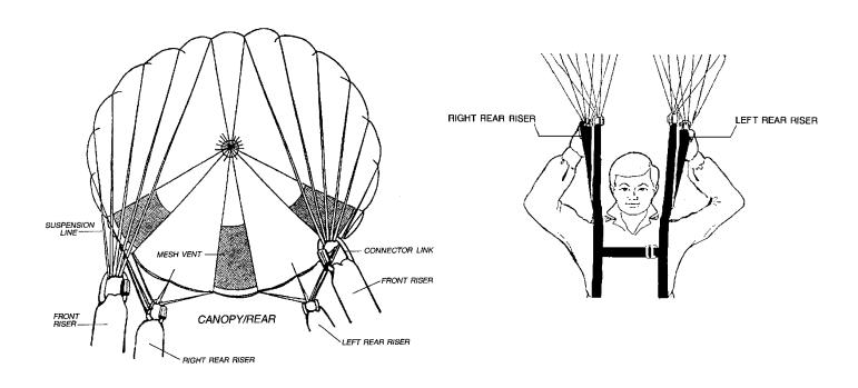
The Parachute can be turned to the right by pulling down the right rear riser 6" to 12", the same applies for a left turn. A rear riser can most effectively be pulled down by placing fingers between suspension lines as they attach to the connector link on the end of the riser. (See diagram above right.) The Parachute will continue turning until the rear riser is released. It takes about 8 - 10 seconds to complete a full 360 degree turn.
