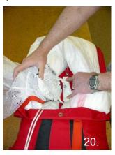
Step 21 - Center the pilot chute on the stiffener base over the S folded bridle.
