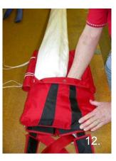
Step 13 - Position the folded canopy up the left side of the container. Bring stiffener cover flap over canopy and use one shot bag to prevent canopy from moving out of pocket.
