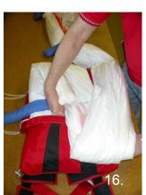
Step 17 - Repeat step #16 until you reach the apex, spread the material from side to side after each fold.
