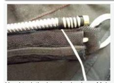
Hand tack the housing in place. Make five turns of hand tack around housing in the direction of the housing channel.
