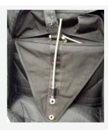
Place new housing with terminal end through drogue loop, positioning the terminal end of housing over original grommet hole.
