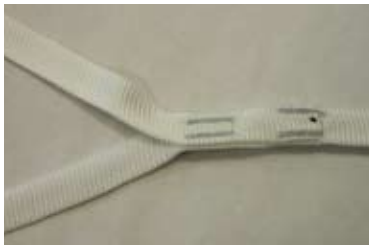
Bartacks secure, tubular in good condition.
