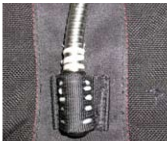
Tacking secure on drogue riser.
