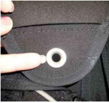
Fingernail doesn't slide under rim.
