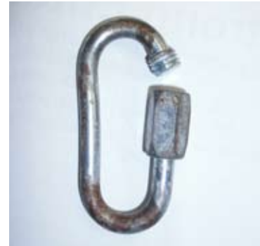
Link bent and rusted.
