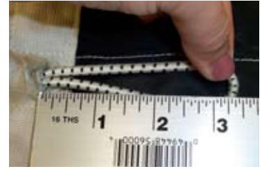
Shock cord loops stretched out. Missing Grommet.
