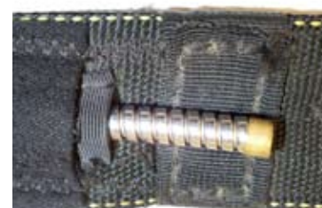
Housing out of place, tacking missing.
