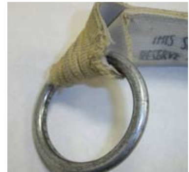
Fraying ring attachment point.
