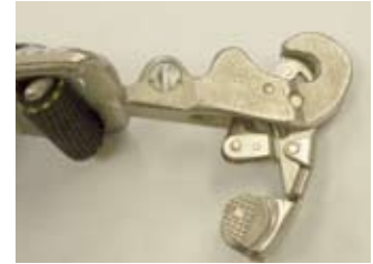
Spring broken, snap stays in open position.
