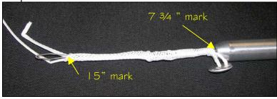
Now insert the finger trap tool in at the  $7 \frac{3}{4}$  " mark and exit at the 15" mark as shown.
