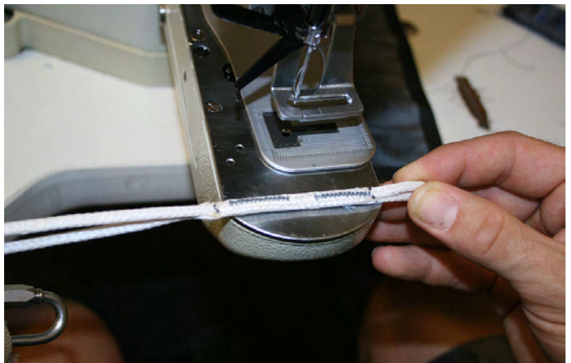
Figure 25. Install Two (2) Bartacks
