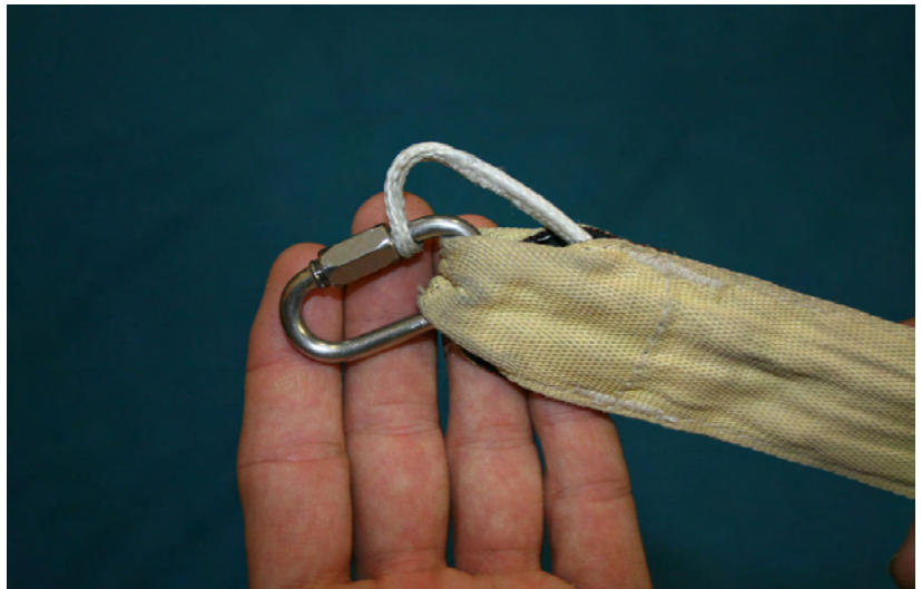
Figure 1. Remove Drogue Bridle from D-Bag
