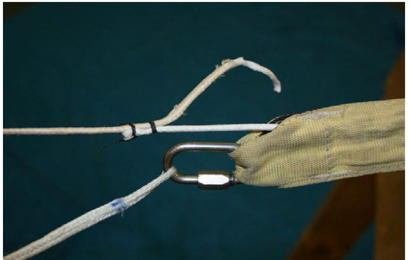
Figure 15. New Centerline Pulled Through
