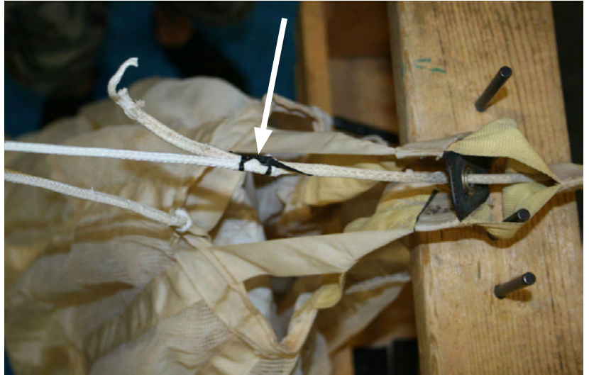
Figure 14. Pull through the New Centerline
