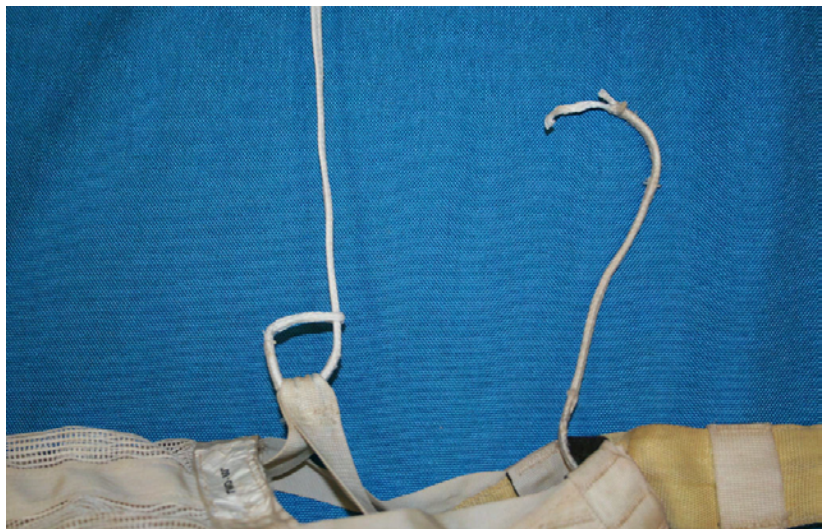
Figure 10. Tie a Lark's Head Knot
