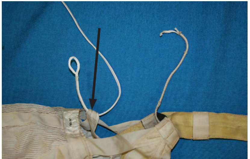
Figure 9. Route the New Centerline
