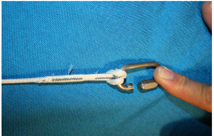
Figure 37. Lark's Head Knot
