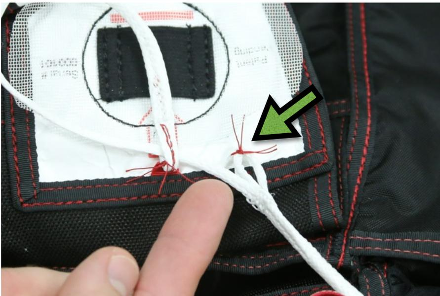
8. Tie the white loop on the Trap Line and the white tab on the Trap together using doubled cotton 24/4 thread. Cut thread leaving ¼" - ½" (.635cm - 1.27cm) tails.
