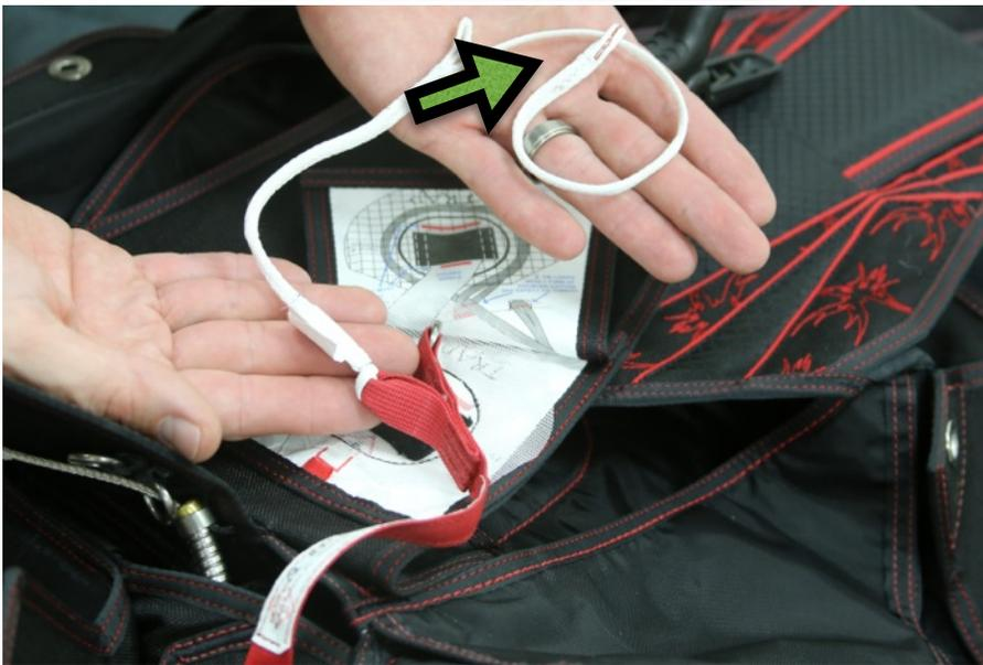
4. Pull the Trap Line through the loop on the end, forming a cinch. The end loop has red stitching.
