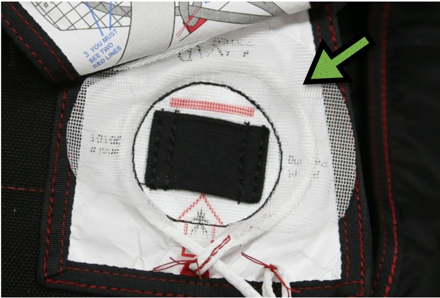
9. **IMPORTANT!** Place the Trap Line **UNDER** the mesh, as shown. The loop should be evenly distributed. Smooth the mesh.
