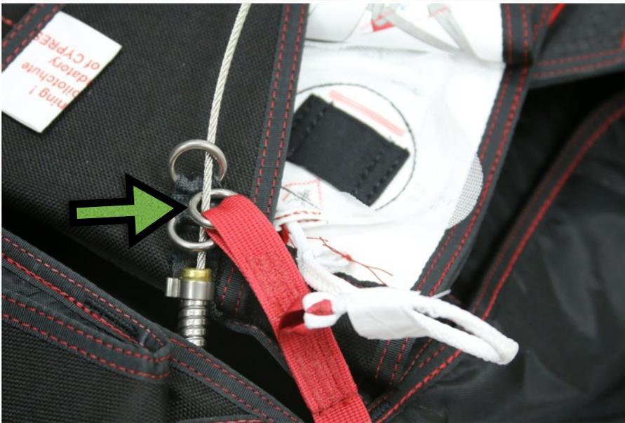
10. With the loop for Trap Line on the RSL facing up, route the ripcord cable through first guide ring on No. 6 reserve pin flap, the ring on the RSL, then the second guide ring on the the No. 6 reserve pin flap, as shown. Make sure that the RSL and Trap Line are not twisted.
