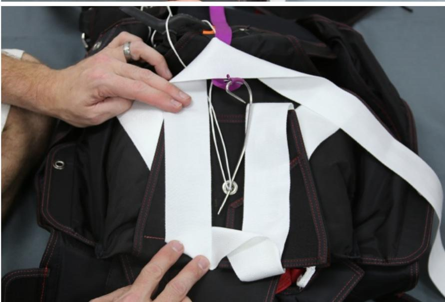
22. Make a short "W" fold placing the remainder of the bridle on the opposite side of grommet. Do not twist.
