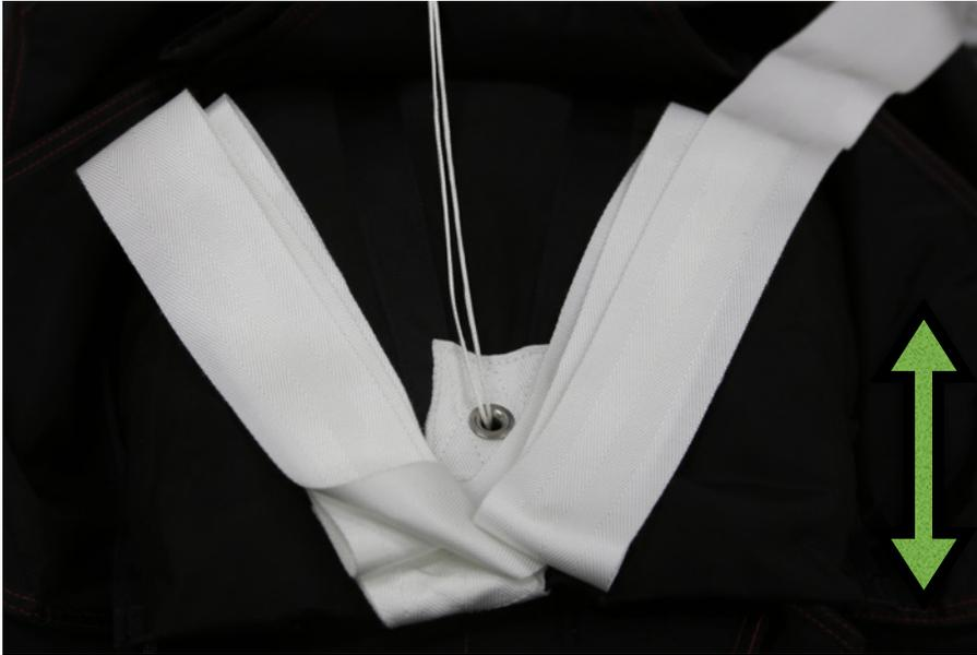
14. Starting on rigger's left, make two stows of the reserve bridle, then make 1-1/2 stows on the right, forming a "V", on top of the packed bag.
