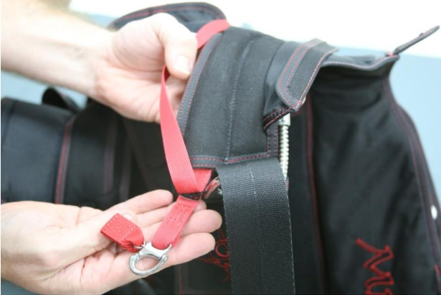
2. Route the RSL over the yoke toward the reserve container and place under the lip of the RSL retainer (a half-twist outward is helpful).
