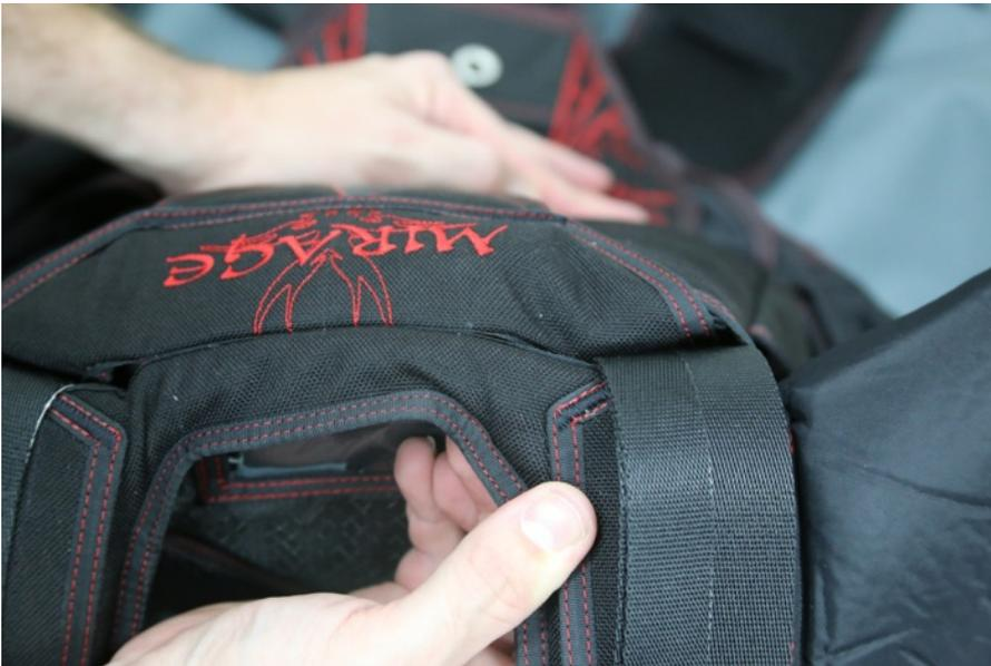
28. When packed, very little (if any) of the Trap System should be visible.
