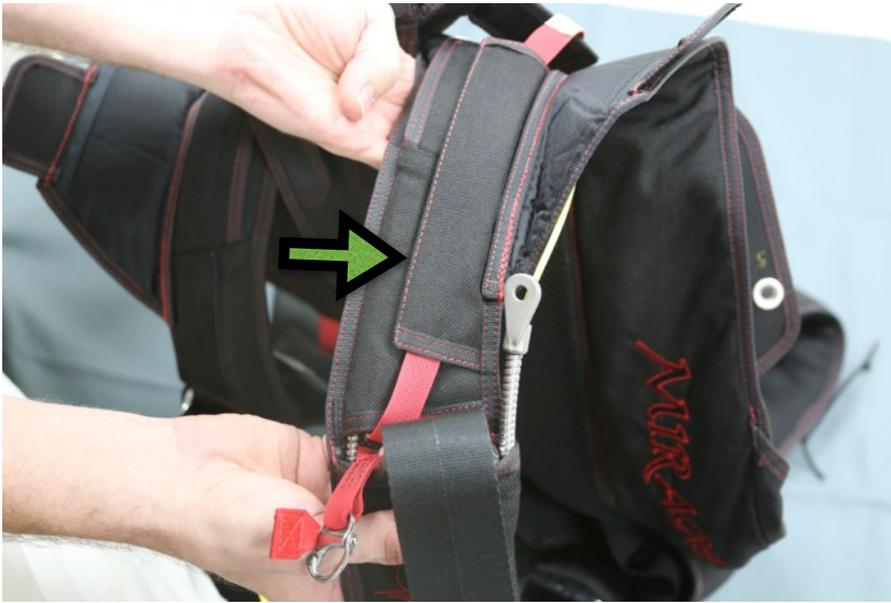
3. Fold the retainer and RSL onto the yoke, removing any twist in the RSL. The label on the RSL should now be facing up.
