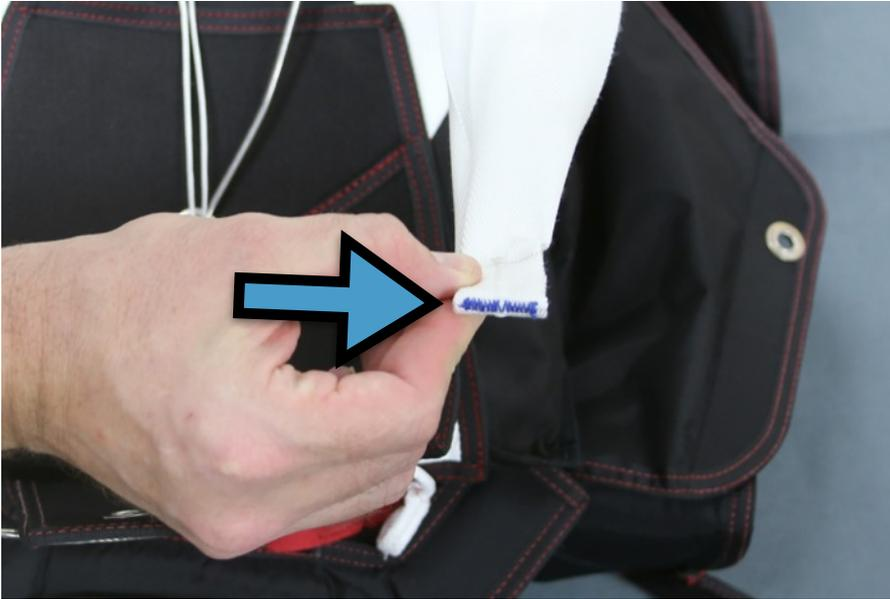
16. Fold the bridle over the No. 1 kicker flap toward the top of the reserve container, removing any twists. Fold the bridle together on the **BLUE** line. The **RED** line should now be facing **DOWN** toward the kicker flap.
