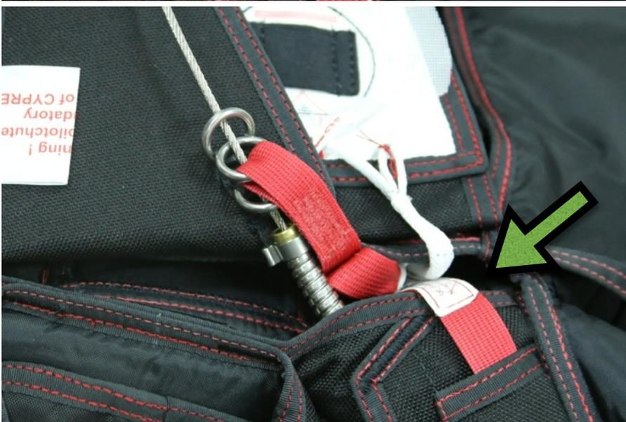
11. Neatly tuck excess RSL and Trap Line between the reserve container and the back pad, as shown. Remove the clamp, if used.
