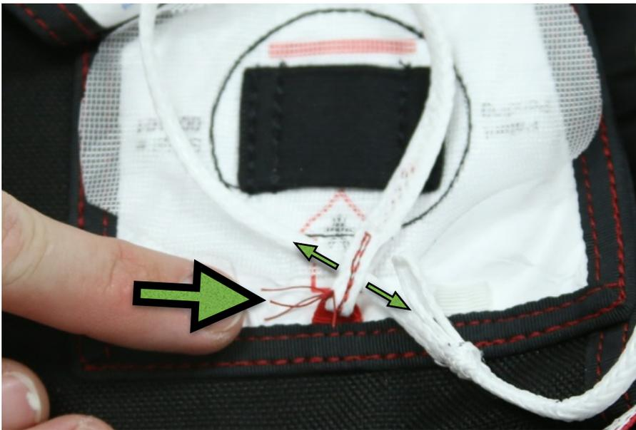
7. Tie the end loop and red tab together with a surgeon's knot and a square knot. Cut thread leaving ¼" - ½" (.635cm - 1.27cm) tails. Make sure that Trap Line is free to slide through the loop after the knot is tied!
