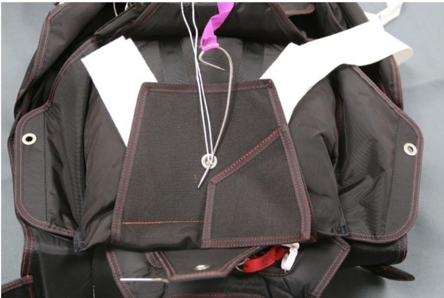
15. Close the No. 1 kicker flap over the stowed bridle with the bridle exiting at the rigger's upper right and pin in place.
