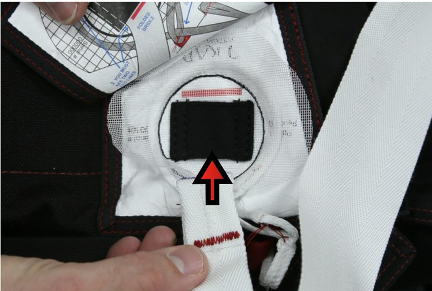
17. Rotate the folded end of bridle under toward the bottom of the reserve container. The **RED** line is now facing **UP** and the remainder of the bridle running to the reserve pilot chute should be **DOWN**. There should be no twists in the bridle.
