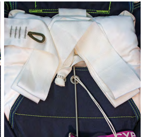
18. Fold bridle in "V" as shown.
