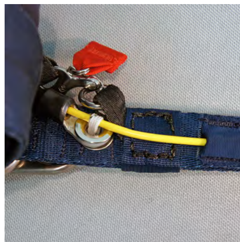
3. Insert the cutaway cable into the Anti-twist Housing.
