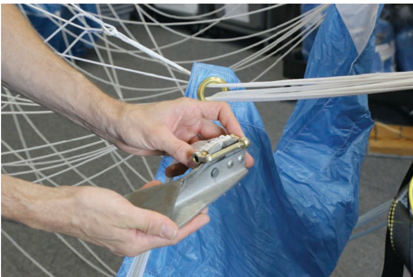
Remove screws and open L-bar using separator tool
