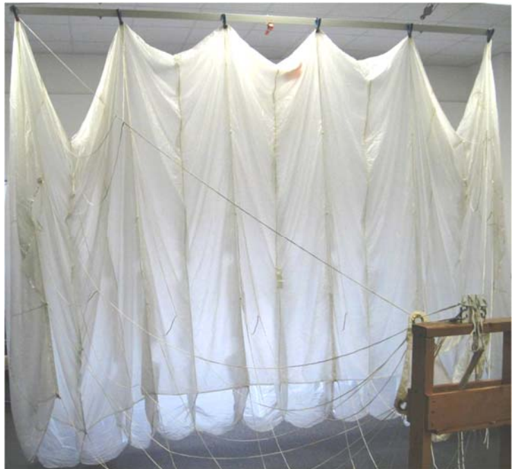
Hanging the canopy by the tail helps in both assembling and inspection.
