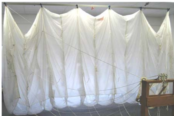
Hanging the canopy by the tail helps in both assembling and inspection.
