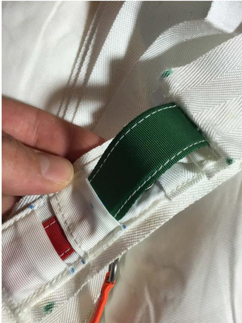
PLACE THE END OF THE GREEN TAB AND ROUTE IT DOWN THROUGH THE SLEEVE, PASS THE CHECK WINDOW, AND SEAT IT INTO THE LOWER PORTION OF THE POCKET.
