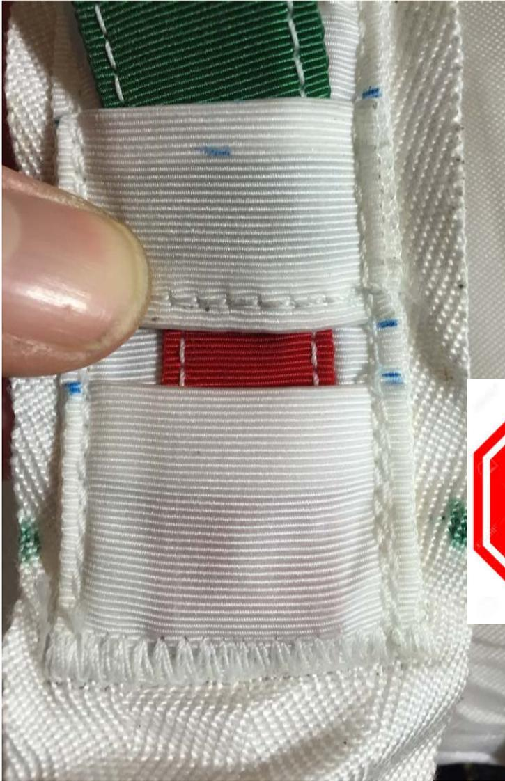
BY SLIDING THE GREEN TAB INTO THE SLEEVE AND PAST THE CHECK WINDOW, YOU ARE PROVIDING THE ABILITY TO INSPECT THE INTEGRITY OF THE PIN SECURITY, ALL THE WAY TO THE LAST FLAP CLOSING
