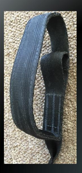
Locate the dive loop area and the top riser loop of the riser.
