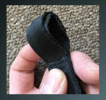
Pinch both layers of Type 17 together about  $\frac{1}{2}$  way back from the top of the loop. (dots indicate pinch location)
