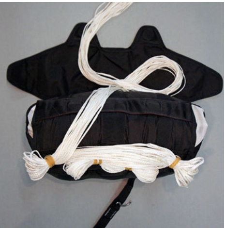
5. Fold the suspension line as shown.
