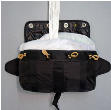
1. Place the main canopy in the D-Bag as shown.
