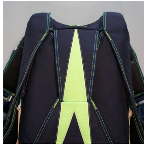
2. Close riser covers over the risers
