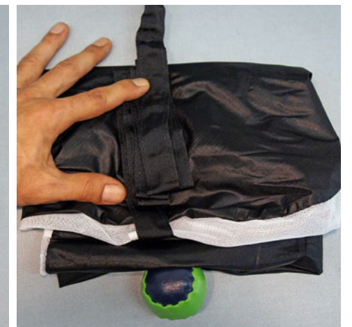
6. Fold excess bridle on top of the pilot chute.
