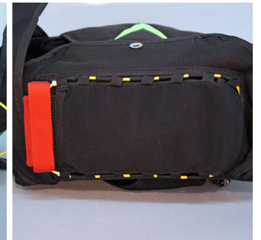
6. Thread yellow cable through loop under Type 12.
