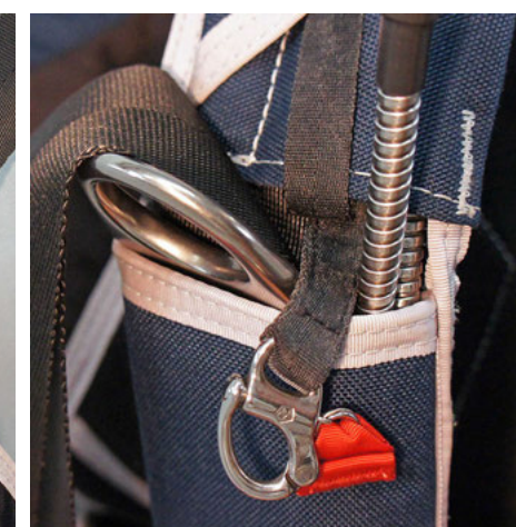
3. Tuck away excess RSL line as shown into the tuck flap and the opening on the yoke.
