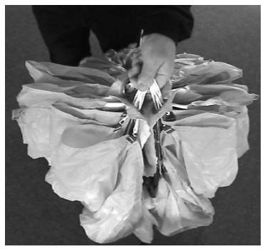
Pick up the center cell by its leading edge (identified by small red tape) and lay it on top of the lines just below the slider. Hold firmly, and make sure that the slider stays in place, pushed up against the slider stops. Also make sure that the steering lines remain in the center and at the back.
