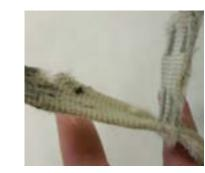
Frayed and worn connecting point.
