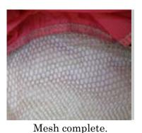
Inspect the mesh for rips and holes.
