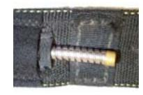
Housing out of place, tacking missing.
