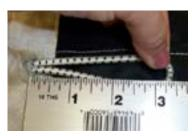
Shock cord loops stretched out. Missing Grommet.
