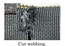
Inspect all webbing on both harnesses for cuts or fraying.
