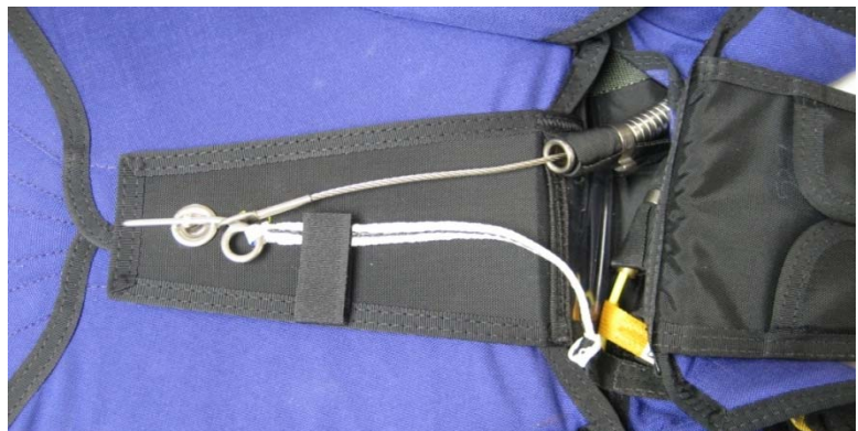
Mate the patch of 5/8" pile hook and loop fastener on the top #6 reserve flap.
