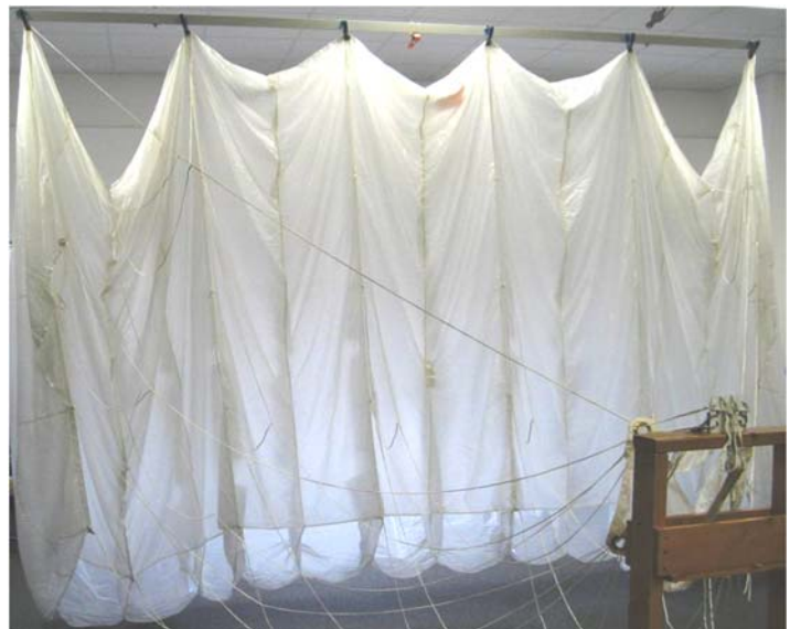
Hanging the canopy by the tail helps in both assembling and inspection.
