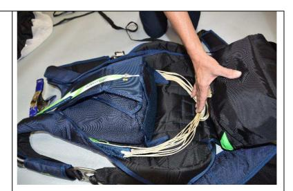
14. Place main deployment bag flat into container with lines stows facing bottom of container and the bridle coming out of the bag towards the bottom of the reserve tray.
