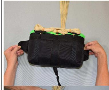
9. Rotate the deployment bag back toward you and tuck magnetic tabs into their magnetic pockets underneath webbing.
