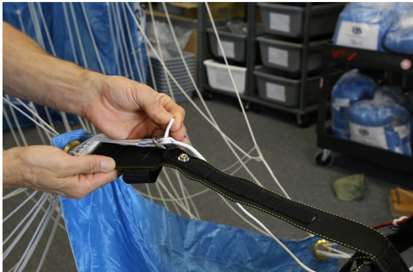
Route Dacron loop through guide ring.
