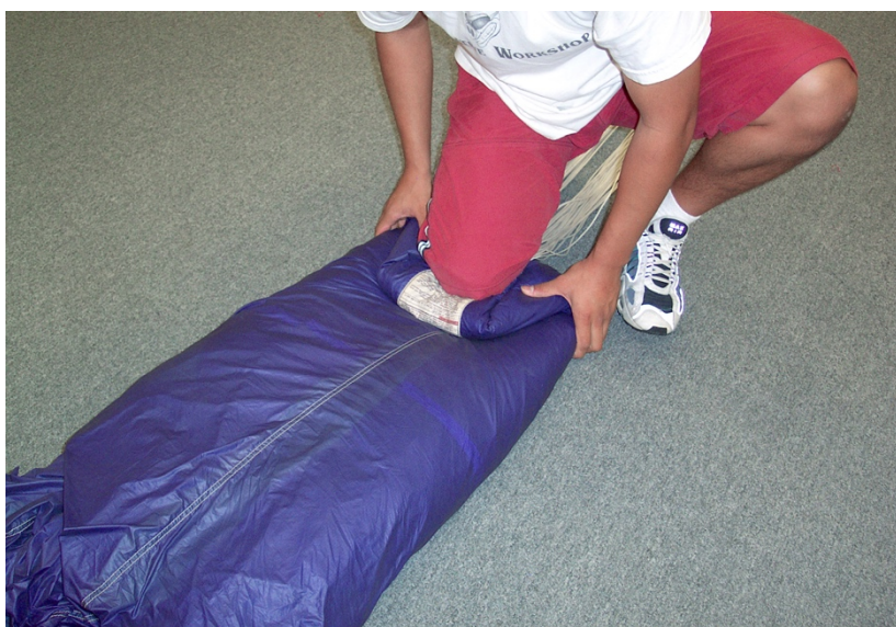
Hold down first S-fold with knee.
