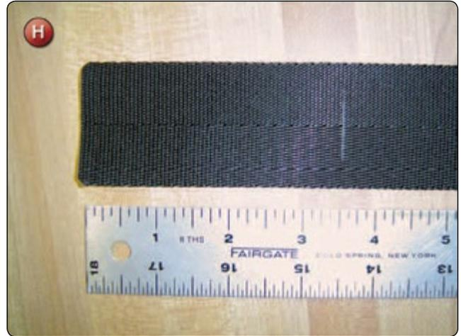
3. Some harnesses are pre-sewn along the edges with a medium duty machine and E thread. If so, duplicate this.
