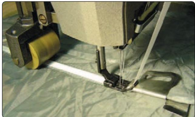
Figure 6-85. Tape feeder and French seam folder.
