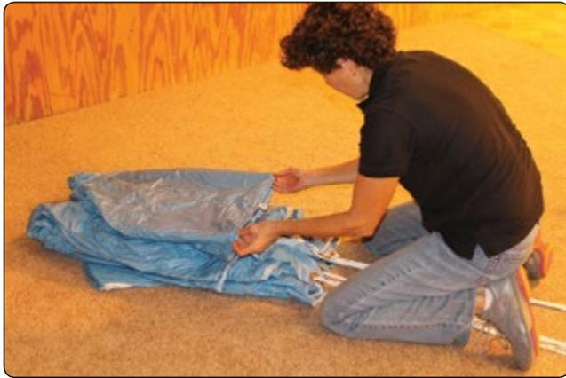
**Figure 5-128.** Without disturbing the rest of the folds, pull the center tail section down to the slider grommets.
