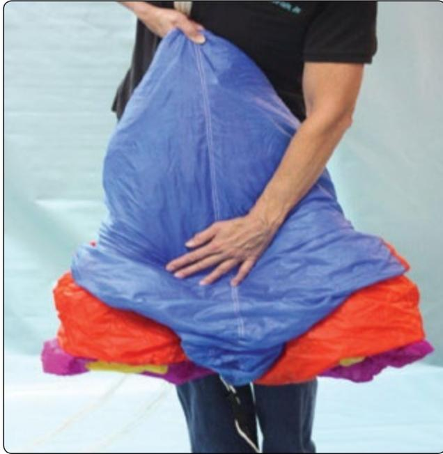
**Figure 4-15.** Press the air out of the canopy.
