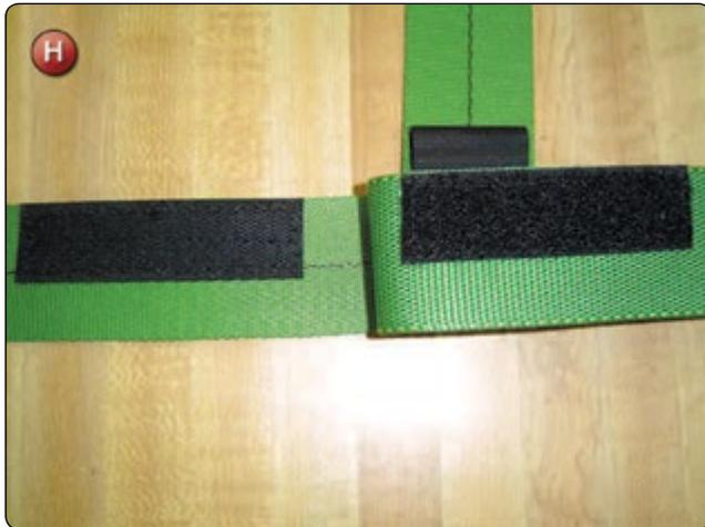
10. Glue the chest strap in place. In this instance, do not forget the housing loop.
