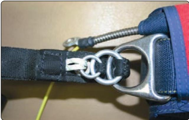
**Figure 4-43.** 3-ring loop over the top ring.
