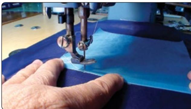
Figure 7-18. Start patch to damage.
