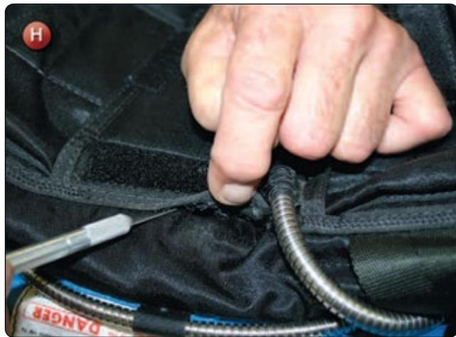
4. Insert the pocket with the mouth towards the channel opening and restitch the container to the backpad. [*Figure I*] Make sure the control head fits into the pocket.
