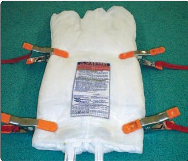
**Figure 5-94.** Finish wrapping tail, four clamps.
