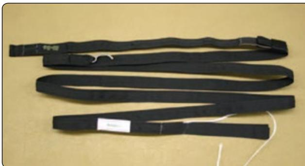
**Figure 2-37.** Kill-line collapsible bridle.
