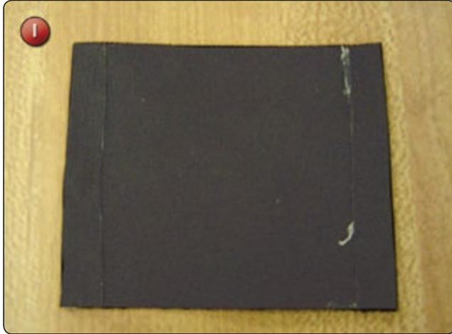
2. Lay the patch in place over the damaged area and mark the corners with a marking pencil. [Figure J]
