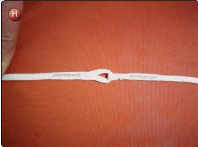
5. Measure and mark the C dimension from the bottom of the brake loop. Run the bitter end of the lower control line through the eyes of two of the upper control lines and finger-trap the line back into itself. Adjust the finger-trap to allow for shrinkage. This completes the non-continuous line method of lower control line fabrication.
