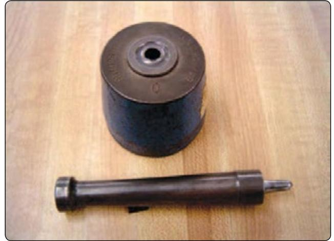
**Figure 6-52.** Size “0” rolled rim spur grommet handset.
