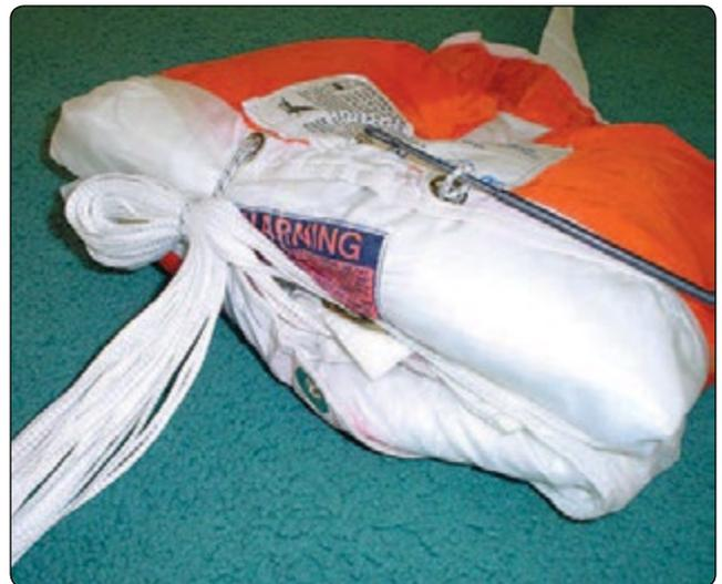
**Figure 5-102.** Close bag and secure locking stows.
