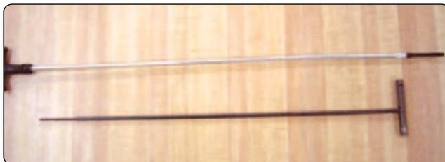
**Figure 6-23.** Pilot chute threading tool.
