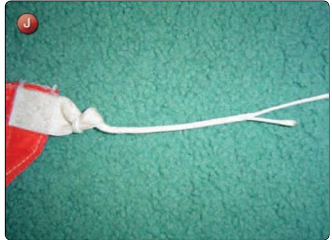
9. Anchor the brake loop securely and apply tension through the complete control line assembly. Measure the dimension A plus B starting at the outside corner of the trailing edge. Adjust the tension of the finger-trap to allow for shrinkage. Pin the finger-trapped section with a marker flag. [Figure K] Repeat with each upper control line until complete.
