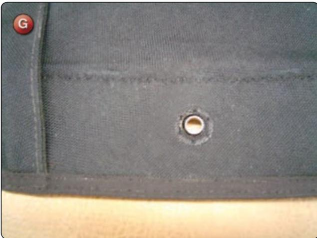
11. Insert the grommet with the correct orientation and set with the grommet set. [Figure H] Make sure that the grommet is set sufficiently so there is no exposed edge to snag the lines or material. Use the feeler gauge to check the gap under the edge of the grommet. [Figure I] It should be no more than .010 inch. If more, hit the set again to tighten the grommet.
