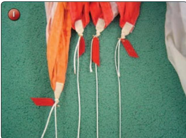
8. Make sure that the lines do not have a twist in them and finger-trap the lines back into themselves with a minimum of a 4 inches finger-trap. Leave the running ends exposed. [Figure J] Do not trim the excess line.
