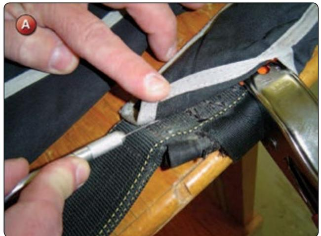
2. Many harnesses have the reserve ripcord housing located on the left side. The housing needs to be disconnected at this location. It is usually secured to a loop located at the chest strap junction. During the
