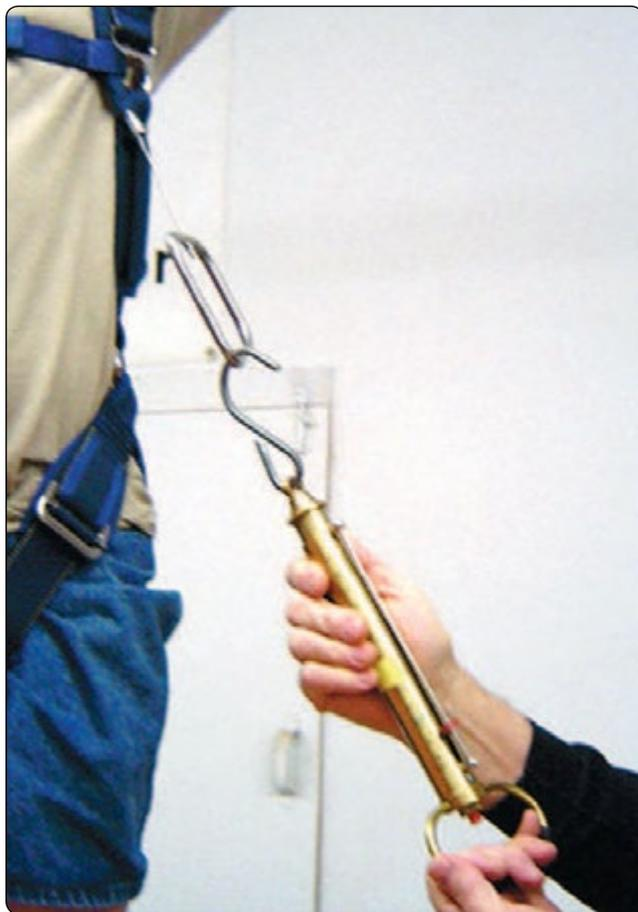
Figure 5-64. Ripcord pull test.
