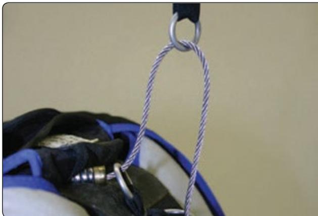
**Figure 2-59.** RSL lanyard extension.
