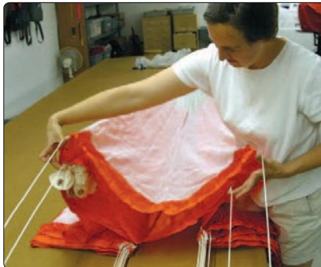
Figure 5-8. Round canopy—four-line check at canopy.
