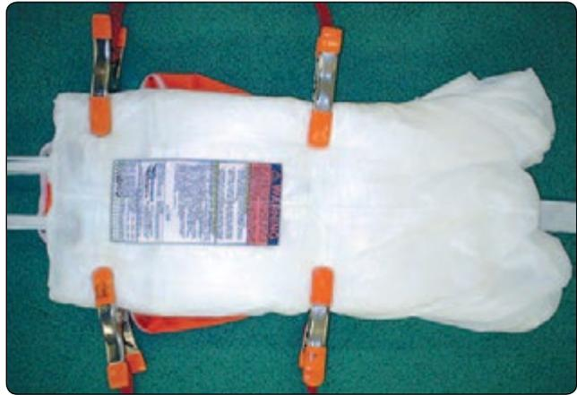
**Figure 5-95.** Bag positioned under canopy.
