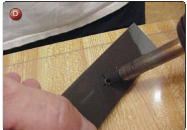
2. Mark out the outline of the original stiffener on the MDS. Mark the center of the hole for the grommet very precisely.
