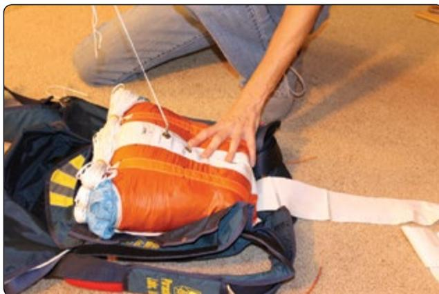
**Figure 5-146.** The bottom bodkin shown in place.
