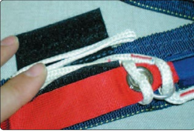
**Figure 5-84.** Set the deployment brakes.
