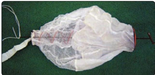
**Figure 5-108.** *Gun rod through the pilot chute.*
