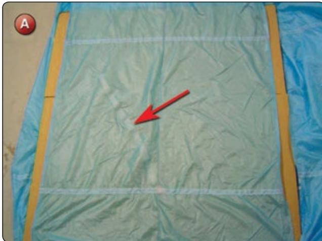
4. Pin the damaged panel to the pin board. Do not overstretch the fabric, but make sure to take all the slack out so the panel is square. In this instance, the canopy had spanwise reinforcing tapes, which were used to stabilize the canopy; however, one of them was damaged and requires replacement. [Figure B]
