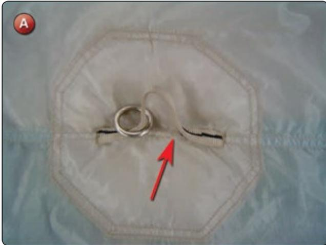
2. If the canopy fabric is damaged, then turn the canopy inside out. The center rib should have a reinforced area that brackets the attachment point. [Figure B]
