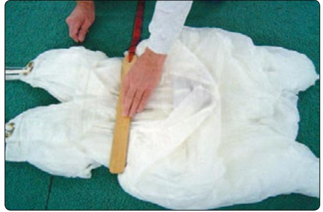
**Figure 5-91.** Packing paddle at 1/3rd location.
