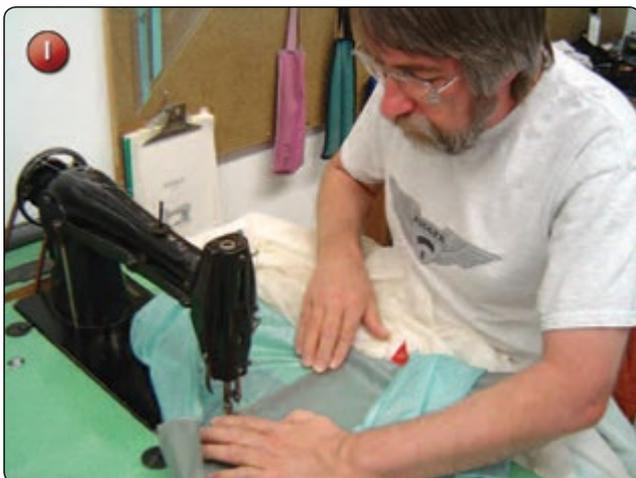
8. Trim the original damaged panel to the trim lines. [Figure J] Fold the fabric under to create a French fell seam. Repeat with the opposite seam. [Figure K]
