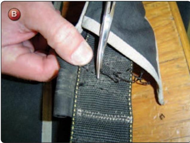
4. Remove the old chest strap webbing from the main lift web. Pay particular attention to the end of the webbing. While most chest straps are installed at right angles to the main lift web, some have an angle cut at the end for better fit. If the webbing has an angle, make sure to duplicate it.
