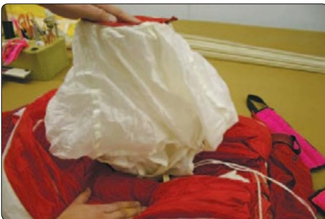
**Figure 4-55.** *Type 1 deployment in a pilot emergency rig.*
