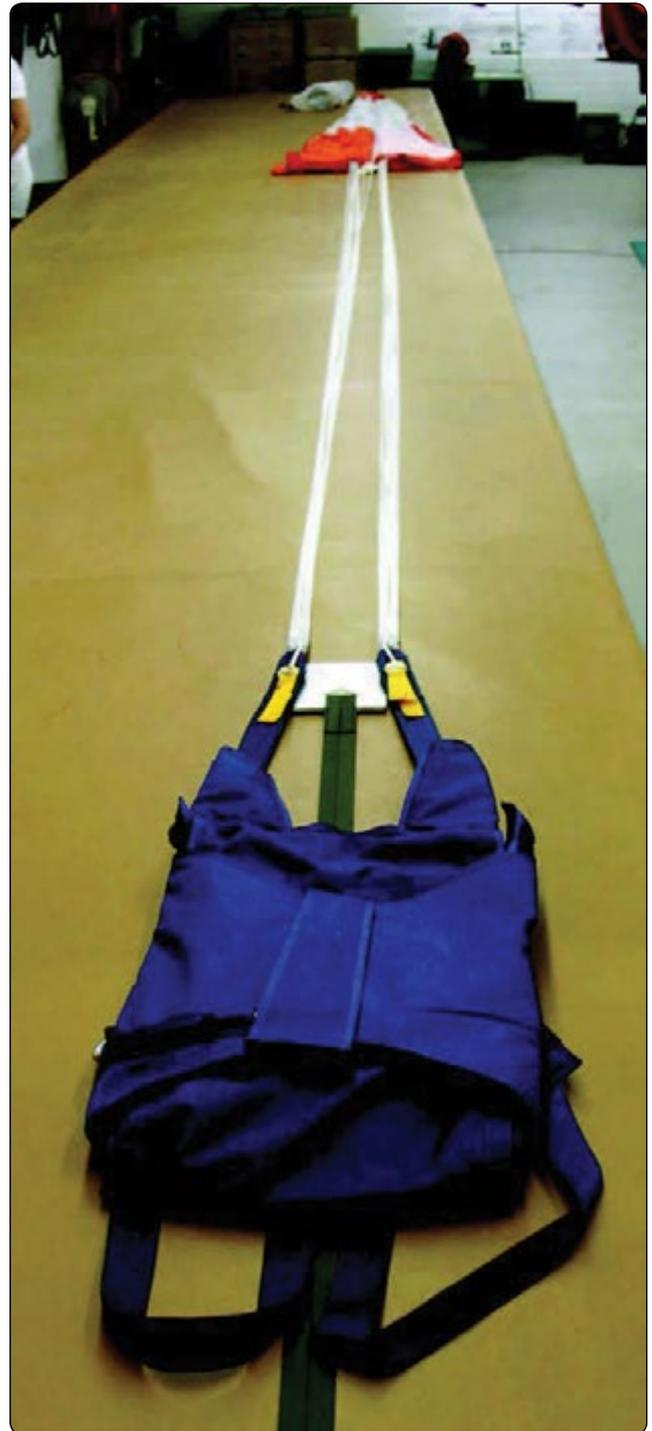
**Figure 5-4.** Round canopy pilot emergency parachute assembly.
