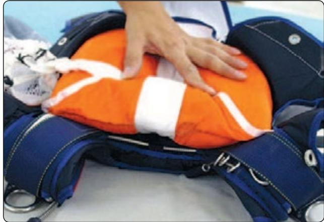
**Figure 5-106.** *Fold the yoke over the bridle.*
