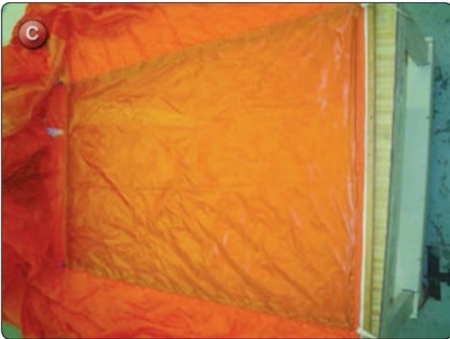
8. Overstitch the end of the cross seam that was left open a minimum of 2 inches and proceed to and down the radial seam and then overstitch the open end of the cross seam. Repeat for the opposite side. It is advisable to hold a bit of tension on the seams as you sew to minimize the shrinkage.
