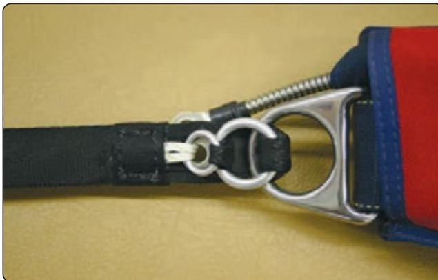
**Figure 4-47.** 3-ring assembled (from front).
