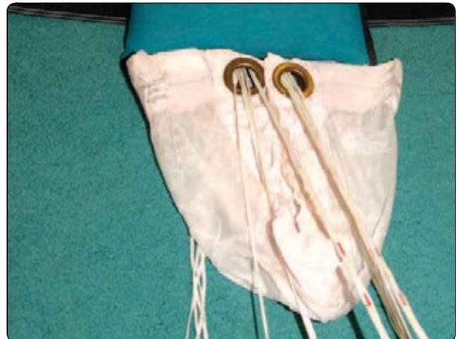
Figure 5-72. Pull slider down.
