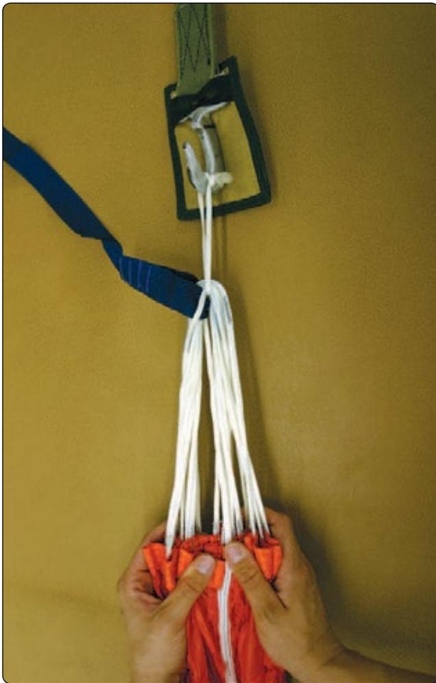
**Figure 5-34.** Straightening the canopy apex.
