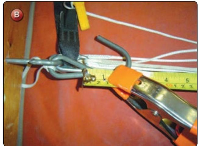
4. Start with the top outside right front corner line of the canopy. This line will be line 1A. Depending on the number of cells to the canopy, on a 7-cell canopy, the left corner line will be line 8A. On a 9-cell canopy, this line will be line 10A. Make sure that the canopy is oriented correctly so that the measurement sequence follows the boxes on the chart.
