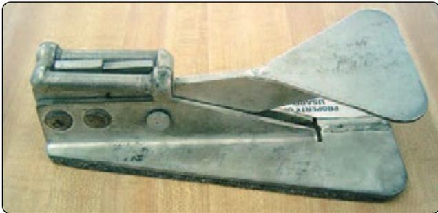
**Figure 6-26.** Connector link separator tool.
