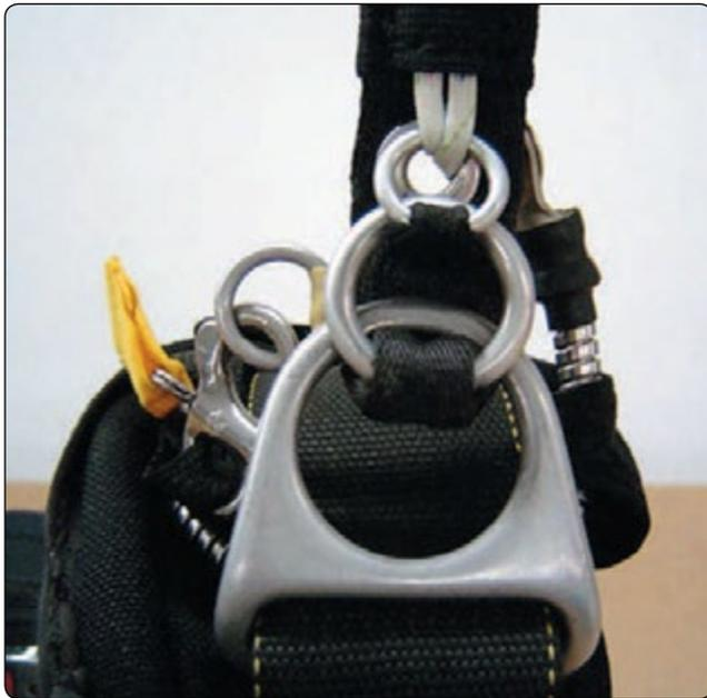
Figure 5-26. 3-Ring<sup>®</sup> release system.
