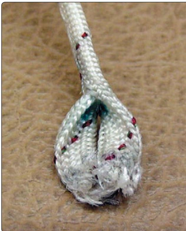
**Figure 5-18.** *Worn closing loop.*
