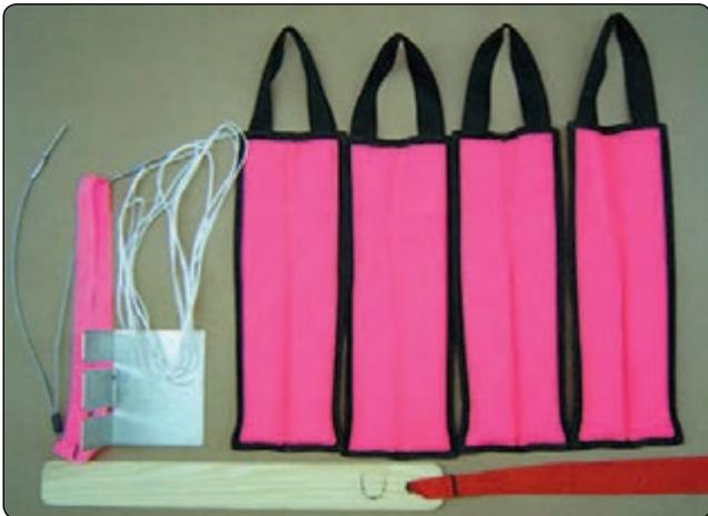
**Figure 5-31.** Round parachute packing tools.
