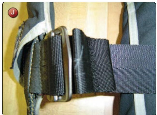
8. If the MLW was attached to the backpad assembly, reattach as per the original configuration. If the backpad is attached in such a manner that does not allow inspection of the back side of the MLW, inspect the stitching at this time before reattaching the backpad.
