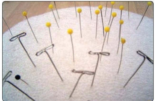
Figure 6-35. Straight and T pins.
