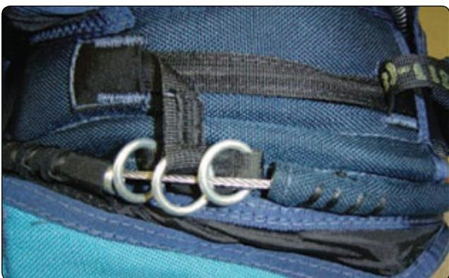
**Figure 2-58.** Ripcord cable routing through rings.
