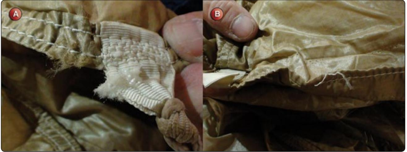
**Figure 7-7.** Line attachment damage.
