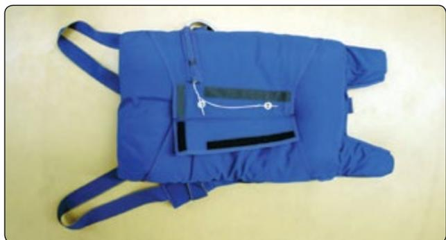
**Figure 5-63.** Ripcord pins in place.
