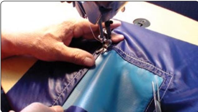
**Figure 7-27.** *Correct fold corner seam.*
