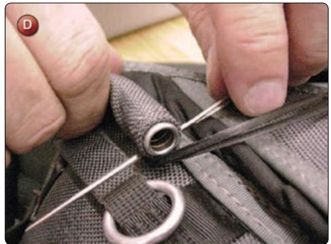
4. Next take the needle and pass it through the top of the channel fabric over the housing. [Figure E]
