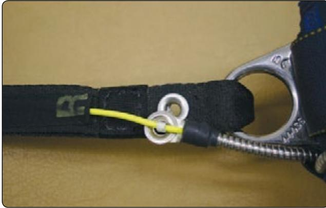
**Figure 4-46.** 3-ring cable through loop.
