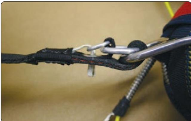
**Figure 4-44.** 3-ring loop profile view.
