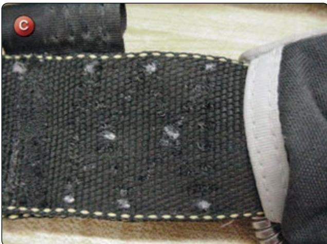
7. If the procedure is a replacement of a damaged chest strap, then it should be replaced to the original length. If so, then remove the rolled stop end so that the finished length may be determined. If the chest strap is to be lengthened, then an appropriate length of webbing needs to be determined. The finished length should be measured from the outside of the main lift web plus 3.50 inches. [Figure D]
