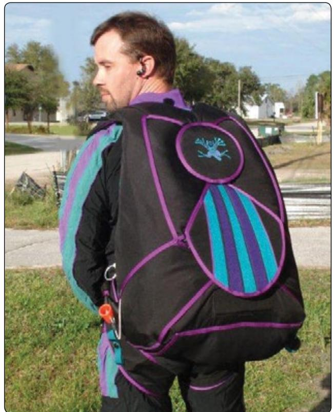
**Figure 2-9.** *Tandem container system.*
