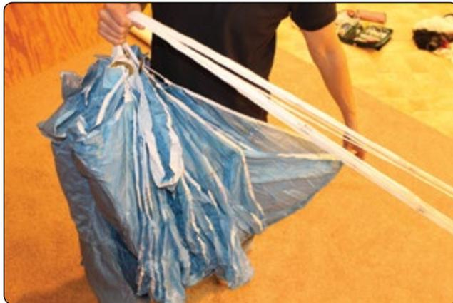
**Figure 5-118.** Flake the nose cells of the canopy.
