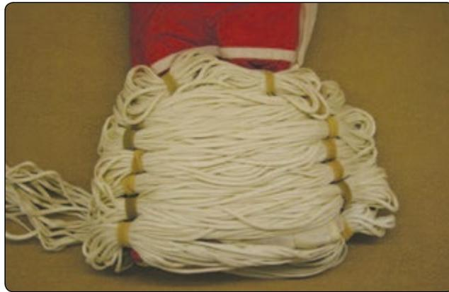
**Figure 2-23.** Type 3 deployment—Phantom canopy.
