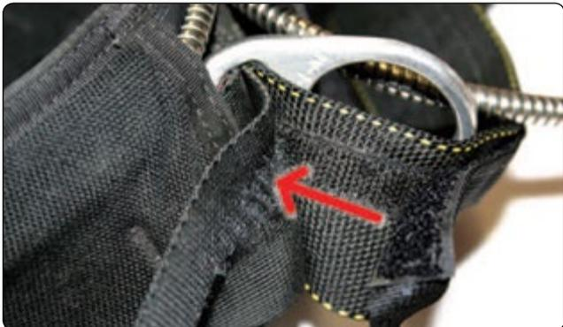
**Figure 2-56.** RSL Velcro riser damage.
