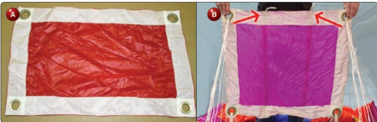
**Figure 2-20.** *A) Non-collapsible slider and B) collapsible slider.*
