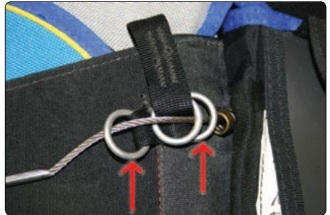
**Figure 2-55.** Double-ring container installation.
