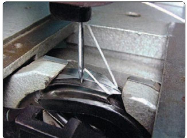
**Figure 6-70.** Second step in forming a stitch.
