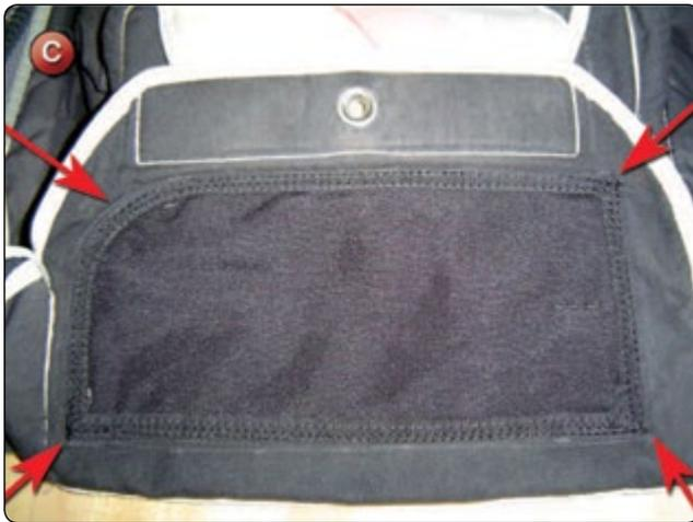
3. Restitch the corner of the main container as per the original configuration.
