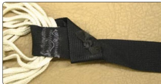
**Figure 2-34.** Hand tack floating bridle loop.
