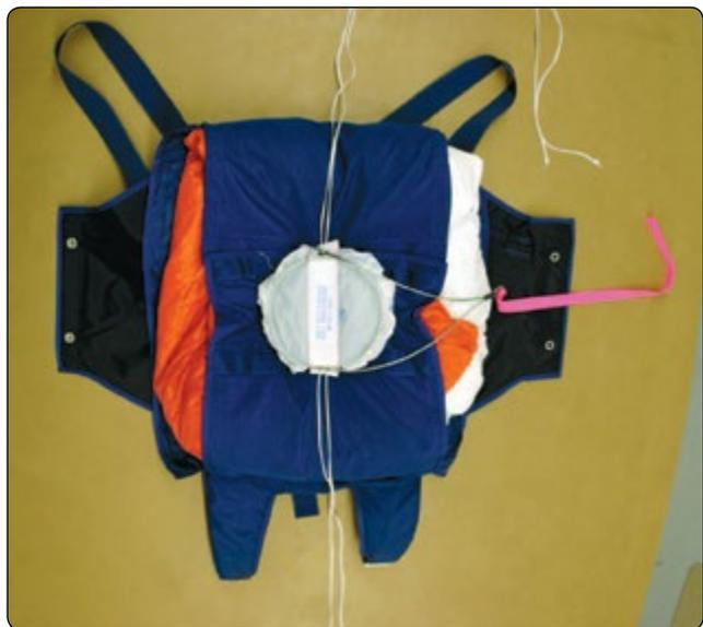
**Figure 5-62.** Pilot chute seated in position.
