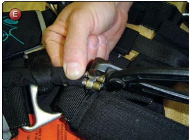
a double clamp to secure the housings together, as well as to the container or pockets. If these are used, inspect the clamp to make sure that it was not damaged when removing the housings and can be reused. Crimp the housings, making sure that the clamp is tight so the housings cannot work loose. [Figure E]
