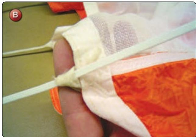
6. Pull the V-tab down until it is even with the rest of the skirt. Mark the line at the edge of the skirt and pin in place. *[Figure C]*
