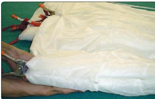
Figure 5-77. Smooth panels under "A" lines.
