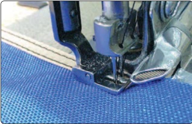
Figure 6-82. Material with binding tape.
