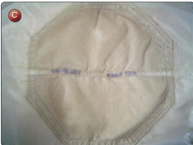
4. Usually the top skin of the cell needs to be repaired. Again, depending on the extent of the damage, either perform a patch on the panel or a partial panel replacement.
