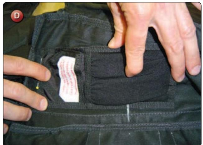
4. Sew around the pocket with the single needle machine. Backstitch .5 inch at each of the corners for reinforcing.
