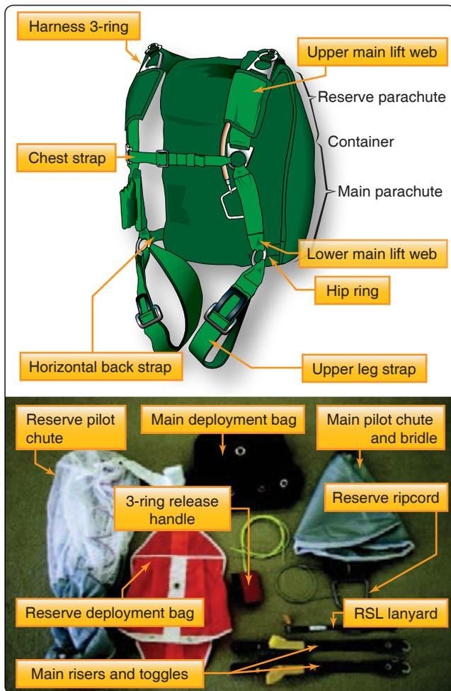
**Figure 2-2.** Subcomponents of the harness/container assembly.
