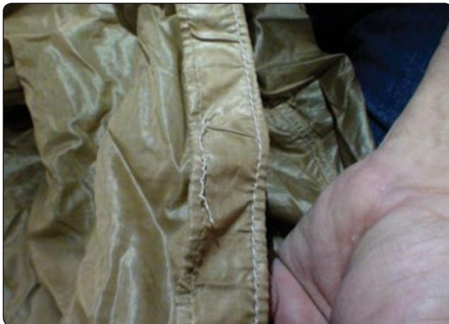
**Figure 7-9.** Long seam damage.
