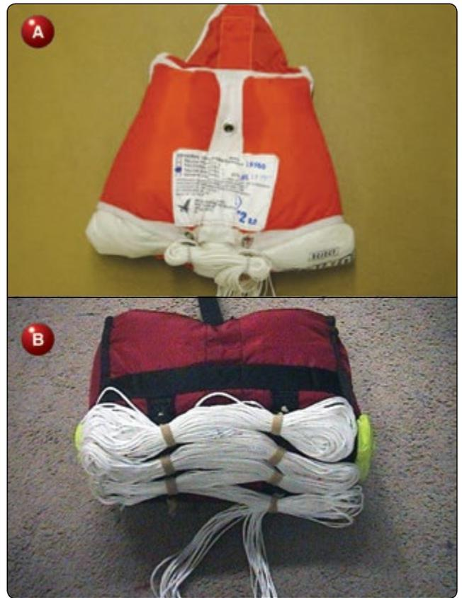
**Figure 2-25.** A) Type 5 deployment—Freebag and B) Type 5 deployment—Speedbag.
