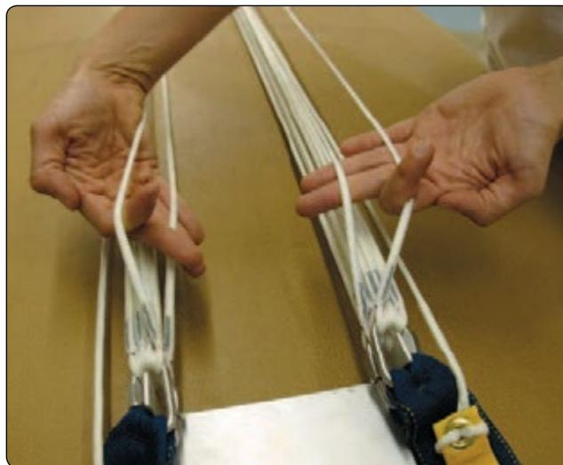
Figure 5-9. Round canopy—four-line check at four-link system.
