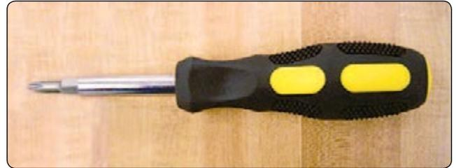
**Figure 6-43.** *Screwdriver—multi-tip.*
