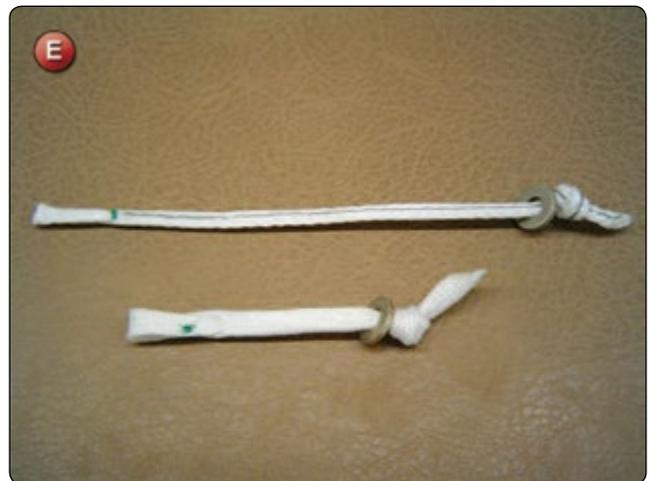
8. If the loop is to be used with a reserve container, it may be required to sew the finger-trapped part of the loop for security. If this is the case, simply sew the length of the finger-trapped portion of the loop with a single-needle machine before hot knitting the end. Start at the running end and sew towards the eye of the loop. Stop sewing approximately .12 inch from the eye and then backstitch a minimum of 1 inch. *[Figure F]* Trim the end with the hot knife.
