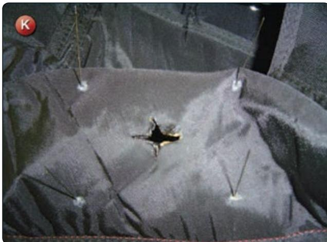
4. If on a main container, take a piece of Type-3 tape big enough to match the outside patch as marked. Cover the inside of the damaged area with the tape.
