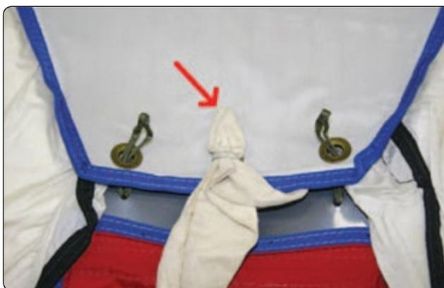
**Figure 2-11.** *Square reserve hesitator loop configuration.*
