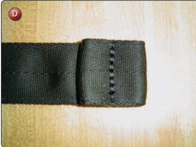
4. Sew the rolled stop end according to *Figure E* with the harness machine.
