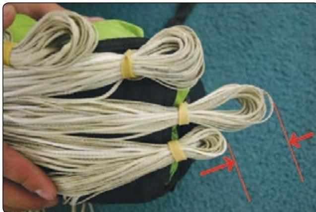
**Figure 4-39.** Line stow length comparison.
