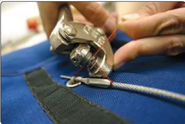
**Figure 5-68.** *Compressing the seal.*
