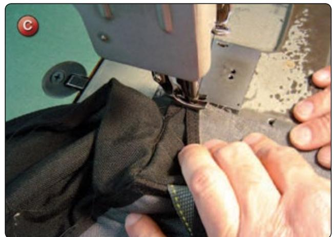
2. If option 1 was used, take the original binding tape, fold over the seam and sew in place with two rows of stitching. Note that there is a second row of stitching sewn directly on top of the inside row of stitching for reinforcement. [Figure D] This is very important.
