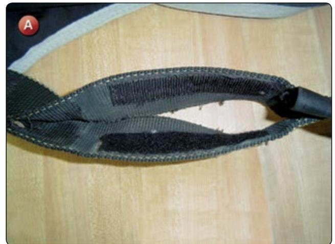
3. Mark the ends of the old Velcro® and remove from the inside of the webbing. Note which side of the webbing the hook and loop are located.
