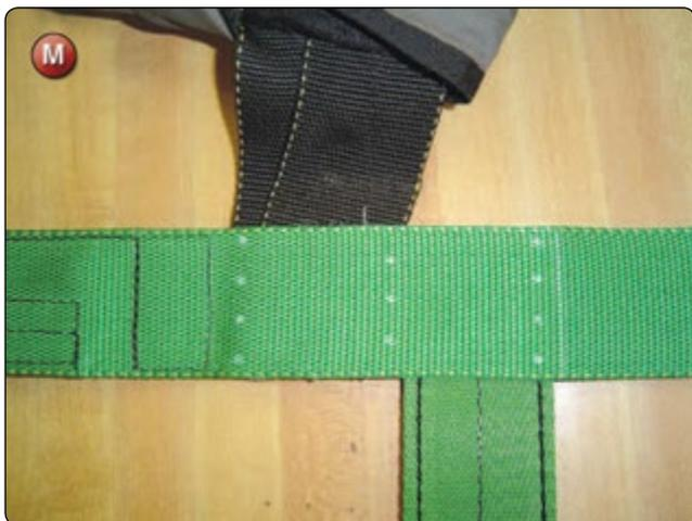
16. Mark the 4-point W-W and then sew with the harness machine. Start the stitch pattern at the front side of the MLW and complete with the over stitch the full length of the pattern. [Figure N] This provides additional reinforcing at the upper leg strap/MLW location.
