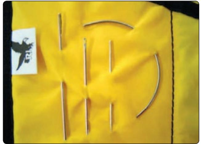
Figure 6-34. Hand tacking needles.
