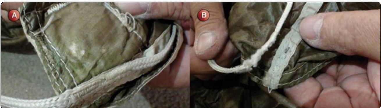
**Figure 7-6.** Stabilizer damage.
