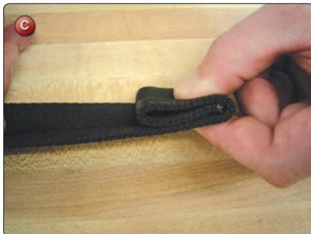
2. Sew the rolled stop end according to Figure D with the harness machine.
