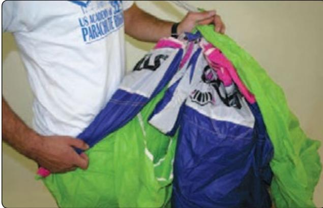
**Figure 4-36.** Rolling the nose of the canopy.
