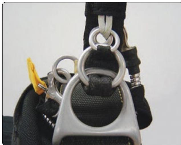
Figure 2-49. Single-side RSL configuration.
