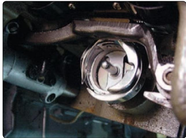
**Figure 6-75.** *Rotary hook.*
