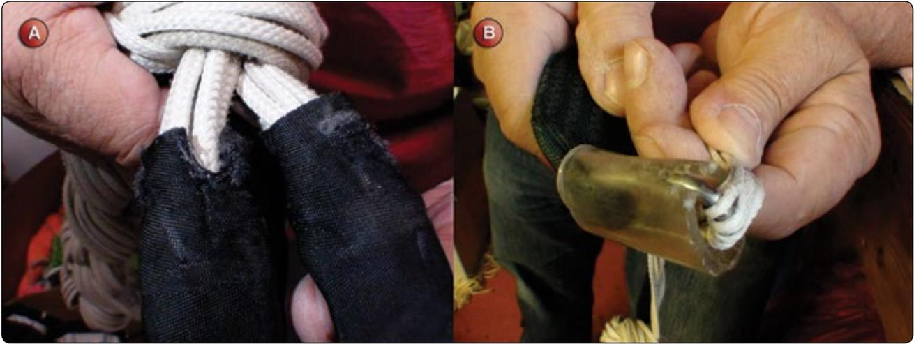
**Figure 7-4.** Protector damage.
