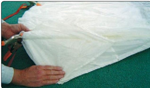
Figure 5-76. Fold half under "A" lines.
