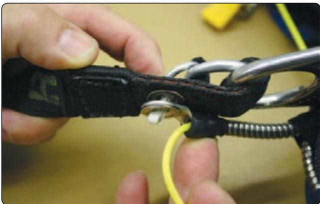
**Figure 4-45.** 3-ring housing terminal over loop (rear).
