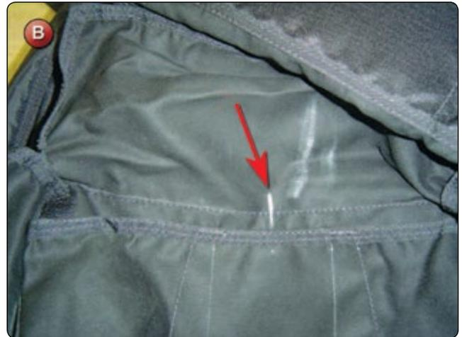
2. Mark the center of the Spandex® portion of the CYPRES® pocket. [Figure C] Do not mark the center of the entire pocket. The Spandex® must be centered on the wall to allow for the correct positioning of the CYPRES® processing unit.
