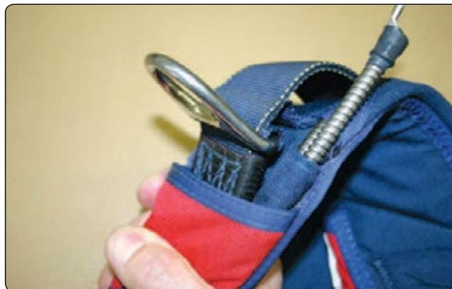
**Figure 4-48.** Harness 3-ring inspection.
