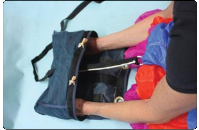
**Figure 4-18.** The “cocoon” should be slightly wider than the deployment bag.
