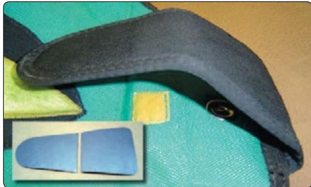
**Figure 5-29.** Main pin protector flap plastic breakage.
