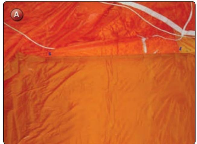
5. Smooth out the panel fabric over the damaged area and align the opposite edge over the opposite cross seam. Cut the panel fabric approximately 1 inch wider than the panel. Fold the edge under and pin in place. You now have the top and bottom cross seams of the panel in place. [Figure B]
