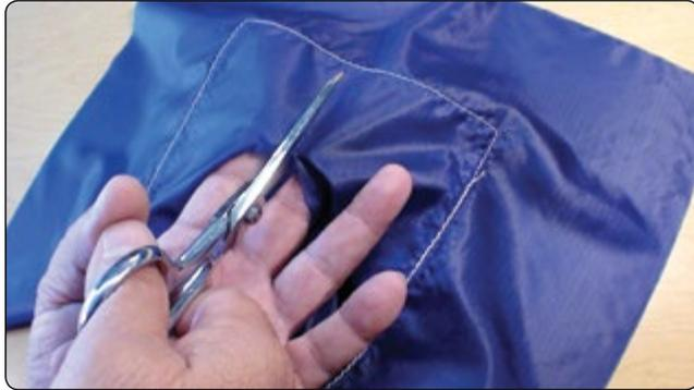
**Figure 7-32.** Wear the damaged parachute as if it were a mitten while cutting and you will not cut the patch that was just carefully placed.
