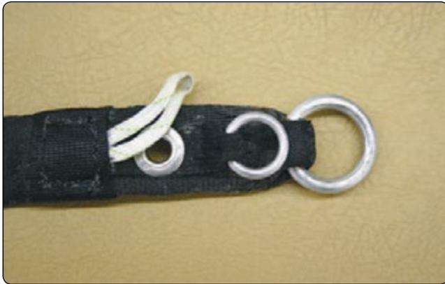
**Figure 4-49.** Riser release end.
