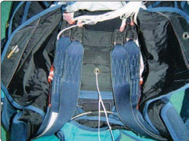
**Figure 5-104.** *Place risers in the pack tray and spread.*
