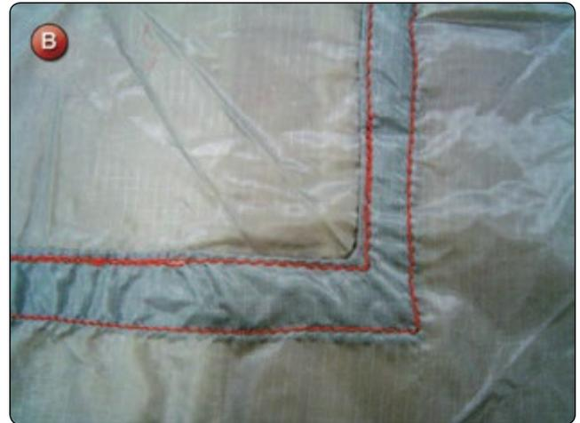
3. If the restitching was done on a radial seam of a round canopy, which has a tape or suspension line within the seam, make sure you did not catch the tape or line in the stitching.
