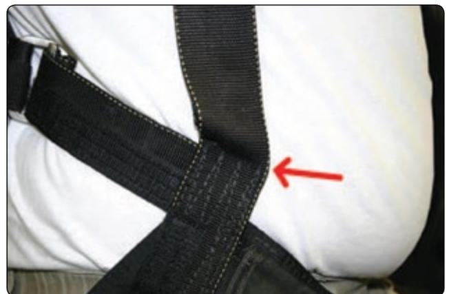
**Figure 2-18.** *Stair-stepped harness (aka stepped harness) junction warping.*
