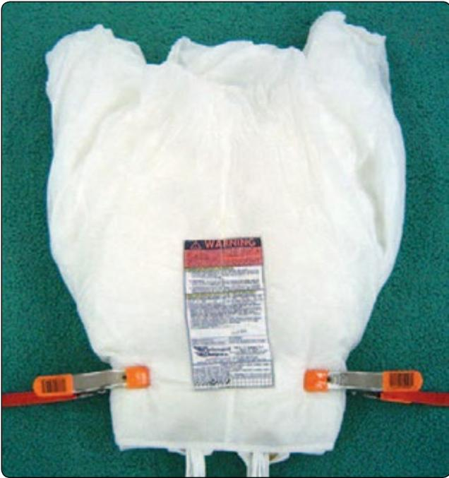
**Figure 5-93.** Wrap tail, two clamps.
