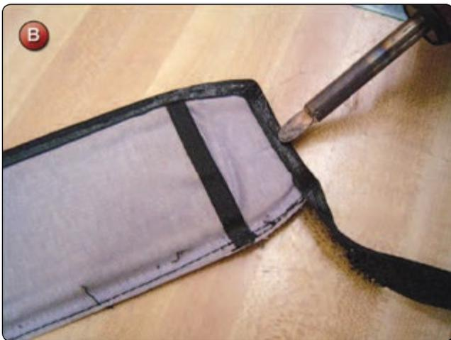
5. Measure the pad and mark. Trim with the hot knife. [Figure C]
