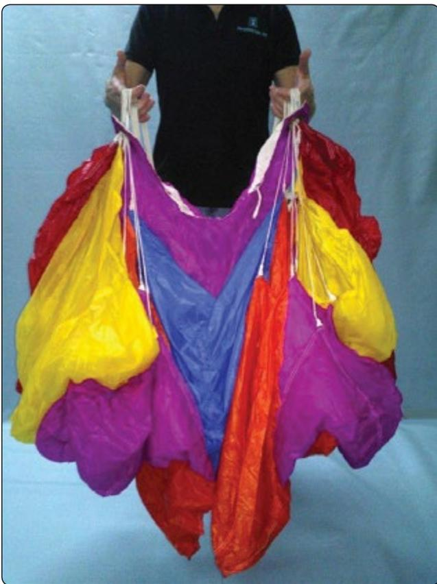
**Figure 4-6.** The nose of the canopy is facing the packer. The tail of the canopy is facing outward.
