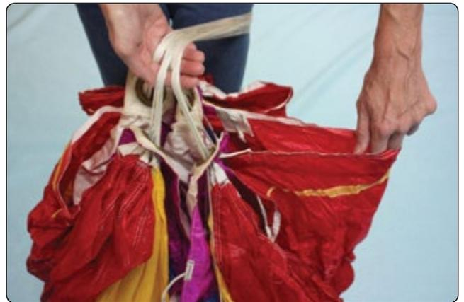
**Figure 4-9.** Flake the canopy fabric between the A-B, B-C, C-D line groups following the perimeter of the canopy.
