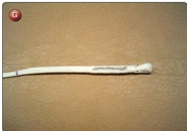
2. Take a second piece of control line material and cut it to the D dimension from *Figure A* plus 12 inches additional. Mark at 6 inches from one end.
