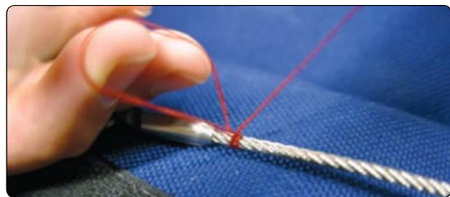
Figure 5-65. Lark’s head the thread on the cable.
