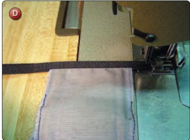
2. Sew the sleeve to the pad and pre-sew the foam with the single needle.
