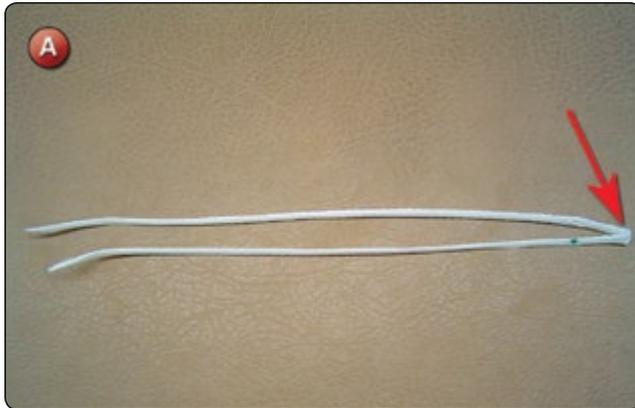
2. Place a mark at 1 inch from the center on the hot knifed end.
