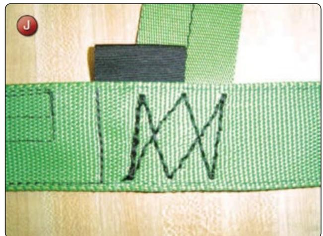
13. Position the 3-ring at the mark on the main lift web and glue in place. Install the Type-12 confluence wrap below the 3-ring and mark the 4-point W-W pattern. [Figure K]
