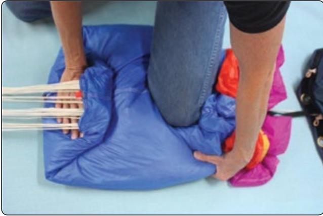
**Figure 4-21.** Make the first “S” fold.
