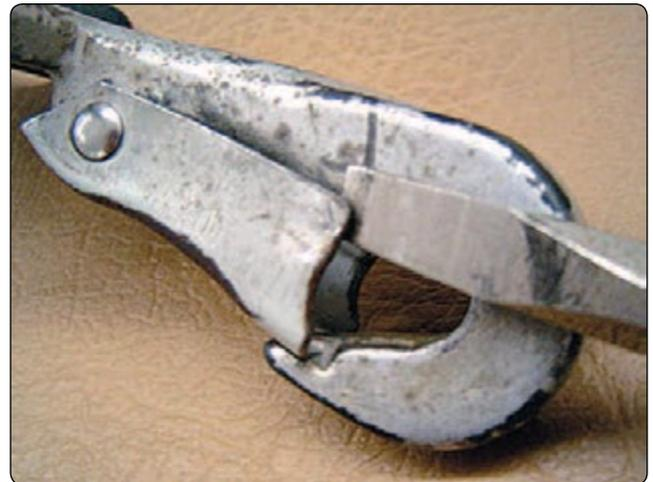
Figure 5-16. B-12 snap gate repair.
