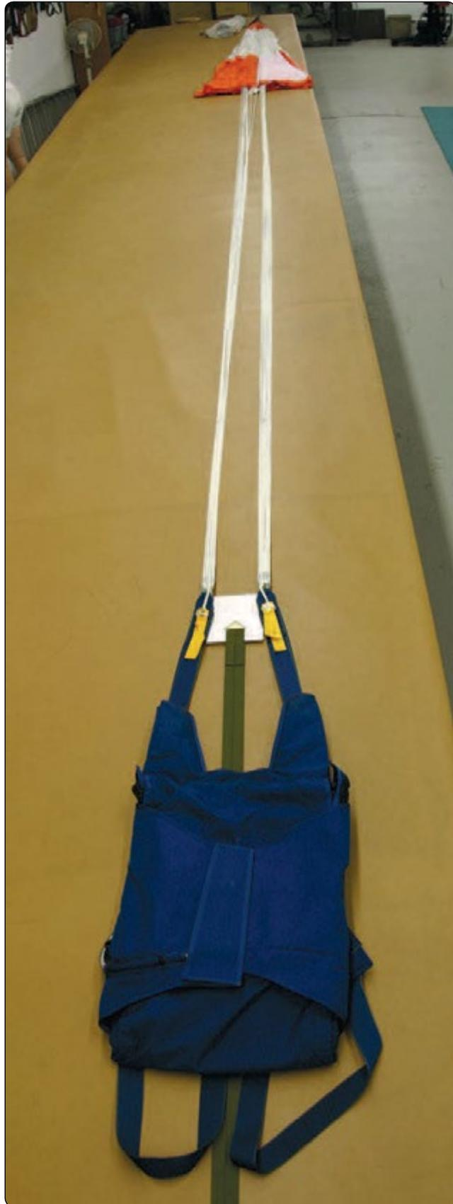
**Figure 5-32.** Round parachute assembly on packing table.
