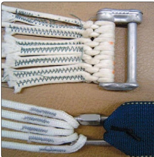
**Figure 5-13.** *Connector link line attachment methods.*
