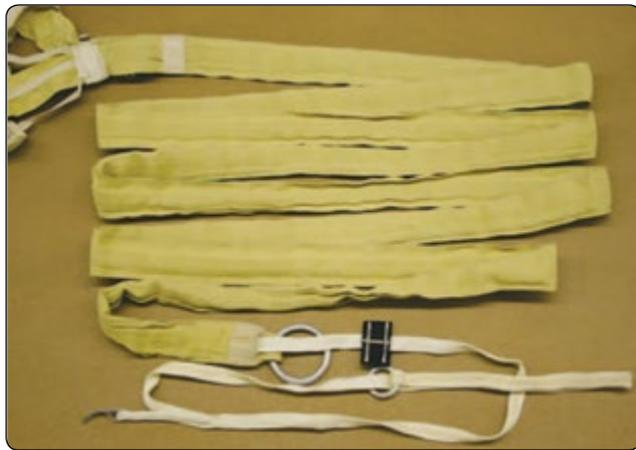
**Figure 2-39.** Tandem main collapsible bridle.
