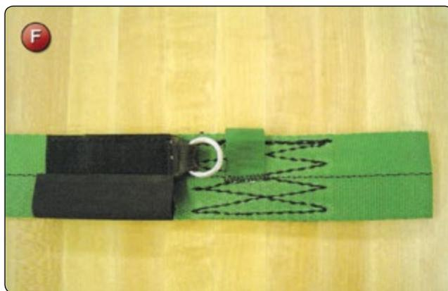
6. If needed, reattach the TSO label at the appropriate location. If the label is the original one and is made from material such as Ty-vek®, try to follow the original needle holes to avoid perforating the material. Too many holes cause the label to tear out.
