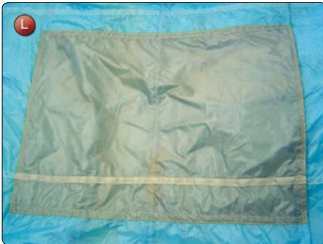
13. If a line attachment has been removed for the repair, the tab must be replaced. Make sure that the line/tab does not have a twist in it. Locate it at the correct location and reattach as per original.
