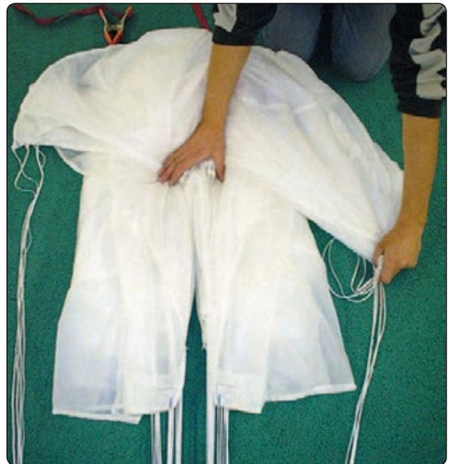
**Figure 5-83.** Pull down the trailing edge.
