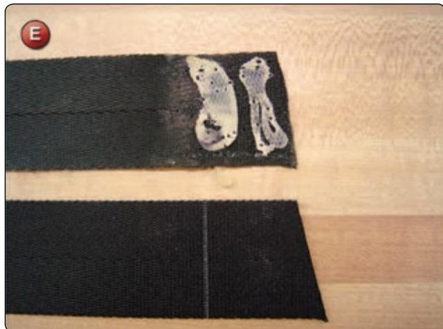
2. Insert the end of the webbing into the MLW junction. Align the end of the chest strap with the outside edge of the MLW. Insert the housing loop back into the junction as well. Lightly glue the MLW to the chest strap. [Figure F] Do not use too much glue.
