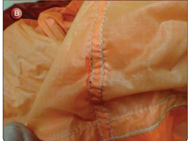
**Figure 7-10.** Fabric damage.
