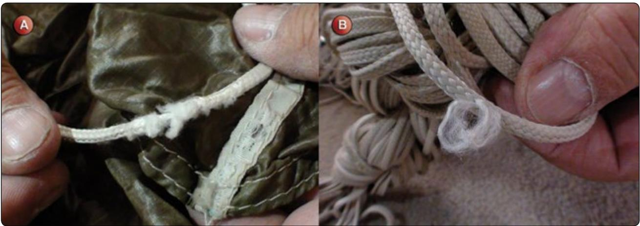
**Figure 7-5.** Line damage.
