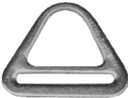
RH44 1 3/4" x 1/4" Slot forged steel, cadmium plated 2,500 lb. proof load Certifies to PS22020 SPECIAL ORDER
