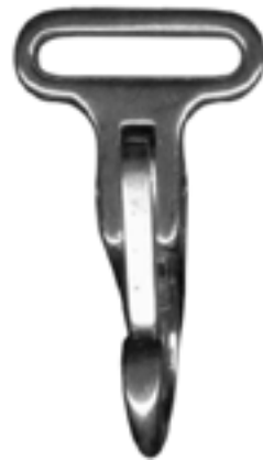
SN704 1" zinc die cast, nickel plated 2 1/2" length for use with DR704-DEE
