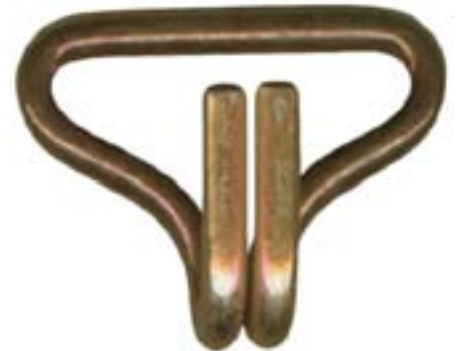
WHK-N/200-2500 Narrow Wire Hook 2" web slot .250" steel wire, yellow cadmium plated 2,500 lb.
