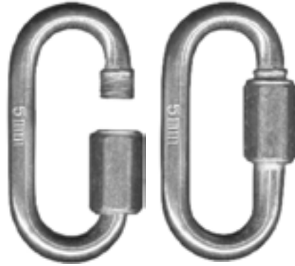
QL51 3/16" steel wire, zinc plated 2" length 1/4" gate opening Use QL66 for Stainless Steel
