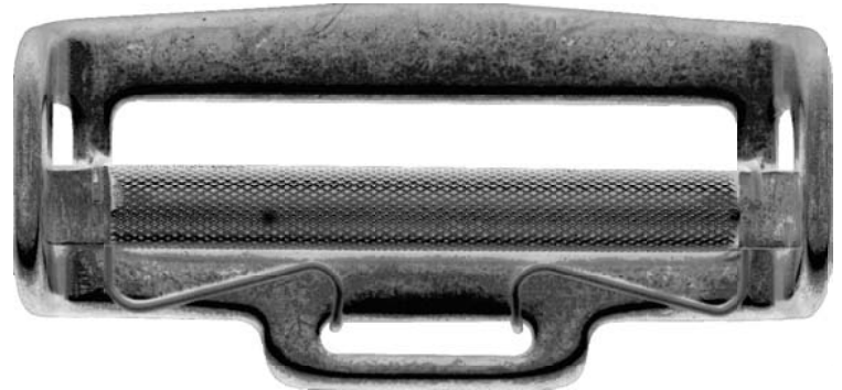
AL16-S Roller Adjuster with Spring Tensioner 3" slot alloy steel, zinc plated 3,000 lb
