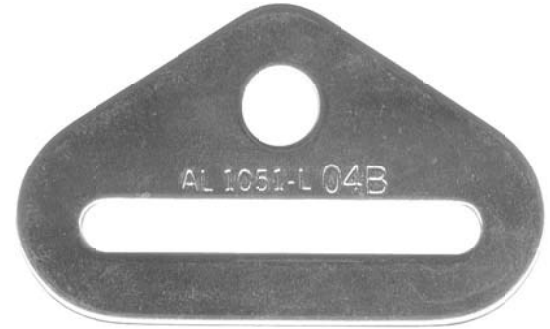
AL1051-L Bolt-In End Fitting 2" x 1/4" slot, 3/8" hole alloy steel, chrome plated 3,000 lb
