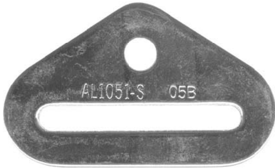
AL1051-S Bolt-In End Fitting 2" x 1/4" slot, 5/16" hole alloy steel, chrome plated 3,000 lb
