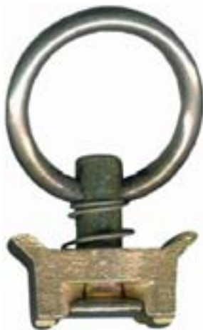
SF17 Single Stud Fitting with 1" O-Ring steel, yellow cadmium plated 4,000 lb. vertical breaking strength
