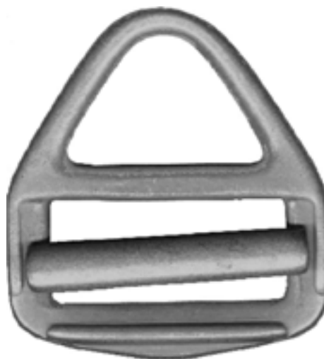
RH17 Adjustable "Reversible Quick Fit" 1 3/4" slot forged steel, cadmium plated 2,500 lb. proof load Certifies to PS70113 SPECIAL ORDER
