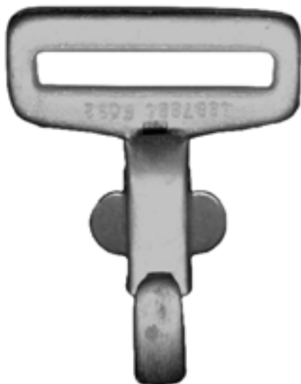
RH98 1 3/4" slot forged steel, cadmium plated 2,500 lb. proof load Certifies to 48B7884 SPECIAL ORDER
