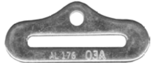
AL176 Bolt-In End Fitting 1 3/4" x 1/4" slot, 1/4" hole alloy steel, zinc plated 3,000 lb
