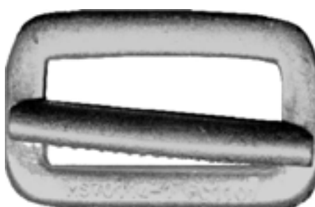
RH10 knurled adjuster bar 1 3/4" x 3/4" forged steel, cadmium plated 2,500 lb proof load PS70114
