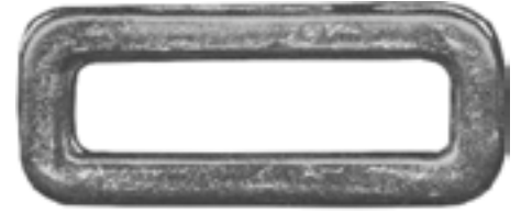
RH7111 Link 1 3/4" x 15/16" flat forged steel, zinc plated 4,000 lb.
