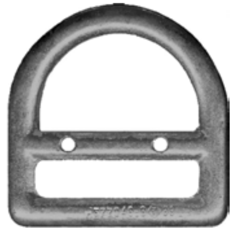
PS28 Slotted D-Ring with holes in cross bar 1 3/4" x 3/8" slot forged steel, cadmium plated Non-certified, surplus version of PS22046-3
