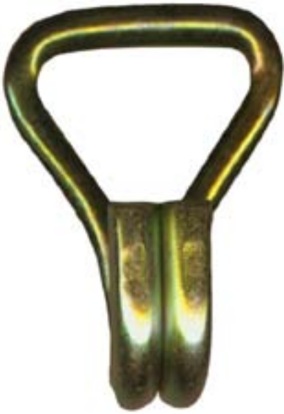
WHK-N/200-5000 Narrow Wire Hook 2" web slot .250" steel wire, yellow cadmium plated 5,000 lb.
