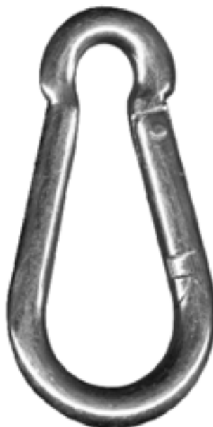
SPC62 5/16" steel wire, zinc plated 3 3/16" length 3/8" gate opening Use SP72 for Stainless Steel
