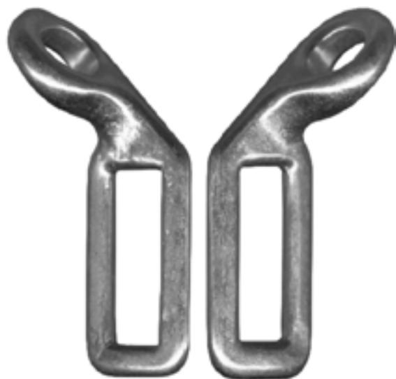
AL55-R & AL55-L Shoulder Links for Latch & Links Left & Right, 1/2" web hole forged steel, zinc plated 3,000 lb
