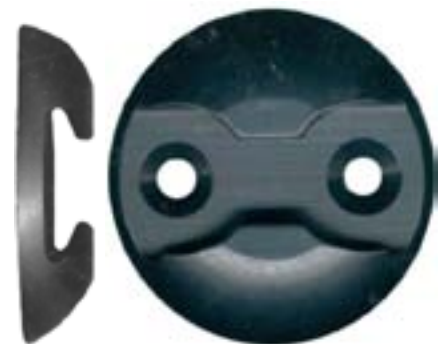
ANCHOR PLATE aluminum, anodized 4,000 lb. vertical breaking strength
