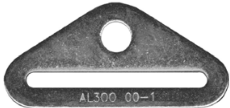
AL300 Bolt-In End Fitting 3" x 1/4" slot, 1/2" hole alloy steel, zinc plated 5,000 lb.
