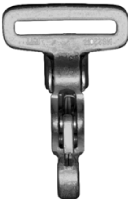
RH101 Harness Ejector Snap 1 3/4" slot forged steel, cadmium plated Certifies to PS22017 SPECIAL ORDER
