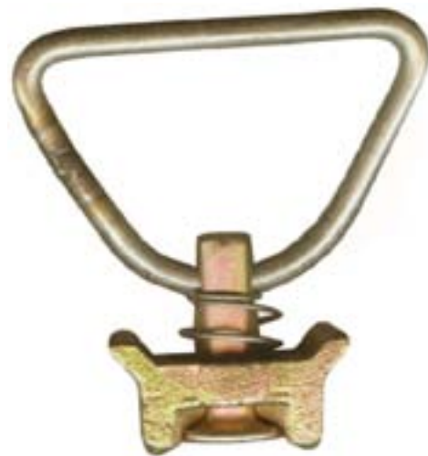
SF18/200 Single Stud Fitting with 2" D-Ring steel, yellow cadmium plated 4,000 lb. vertical breaking strength
