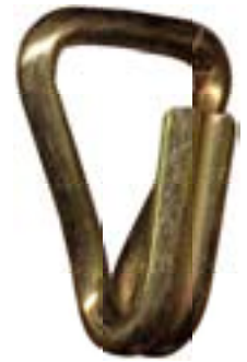
WHK-N/100-500 Narrow Wire Hook 1" web slot .190" steel wire yellow cadmium plated 500 lb.
