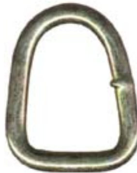
DR/100-5000 Cargo D-Ring 1" x 1 5/16" welded .250" steel wire yellow cadmium plated 5,000 lb.
