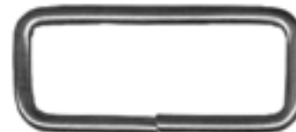
LP4950 Non-Welded Loop 1 1/2" x 1/2" .120" steel wire, nickel plated
