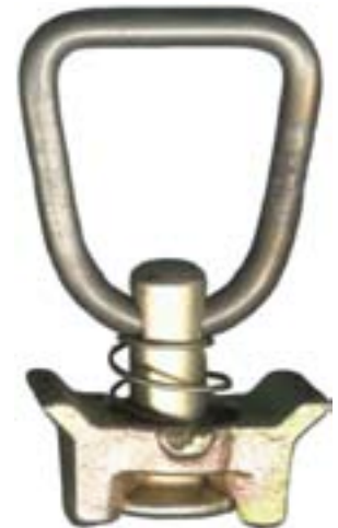
SF18/100 Single Stud Fitting with 1" D-Ring steel, yellow cadmium plated 4,000 lb. vertical breaking strength
