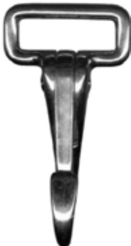
SN703 1" zinc die cast, nickel plated 2 1/2" length
