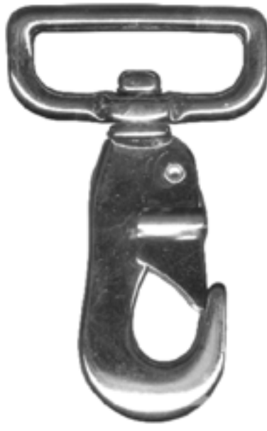
SN848-S 1 1/2" zinc die cast, nickel plated 3 1/8" length
