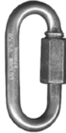
QL52 1/4" steel wire, zinc plated 2 1/4" length 9/32" gate opening Use QL67 for Stainless Steel
