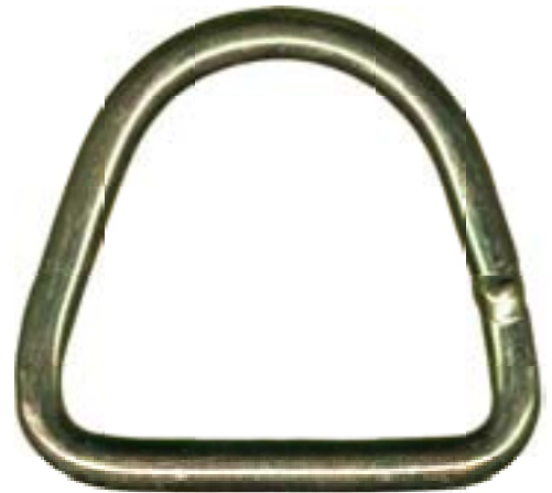
DR/200-5000 Cargo D-Ring 2" x 1 13/16" welded .250" steel wire yellow cadmium plated 5,000 lb.
