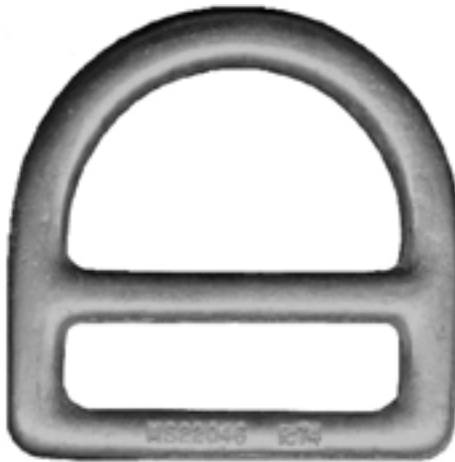
RH27 Slotted D-Ring 1 3/4" x 3/8" slot forged steel, cadmium plated 5,000 lb proof load Certifies to PS22046
