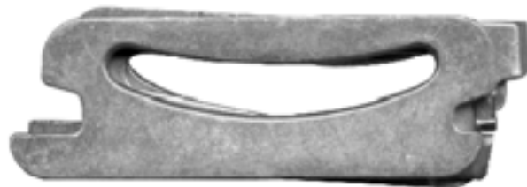
ET/200 E-Track Fitting - 3-Piece 2" web slot steel, yellow cadmium plated 3,000 lb.
