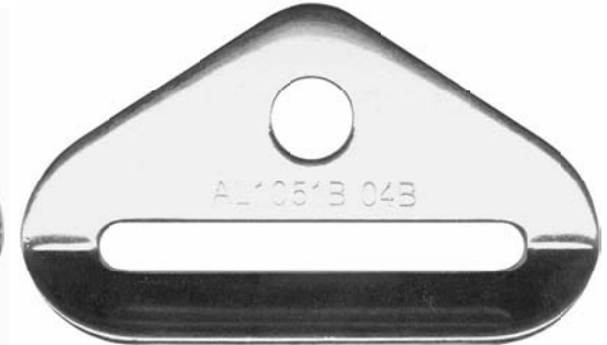
AL1051-B Bolt-In End Fitting 2" slot x 1/4", 3/8" hole, 45° bend alloy steel, chrome plated 3,000 lb
