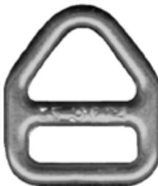
AL45/100-ZINC 1" x 3/8" slot forged steel, zinc plated 4,000 lb.
