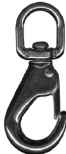
SN92 5/8" zinc die cast, nickel plated 3 1/4" length
