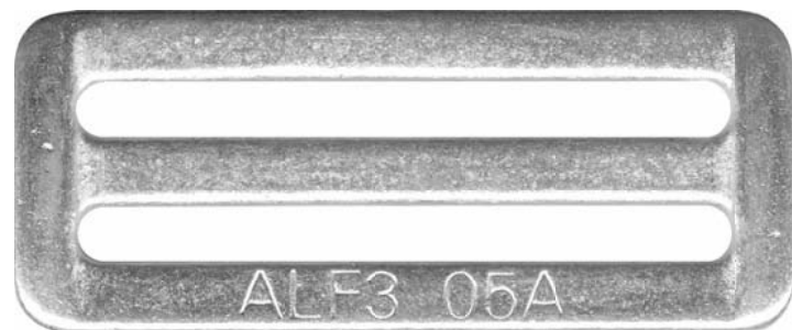
ALF3 3" x 1/4" slots forged steel, zinc plated 5,000 lb.
