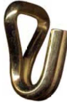
WHK-N/100-3000 Narrow Wire Hook 1" web slot .250" steel wire yellow cadmium plated 3,000 lb.
