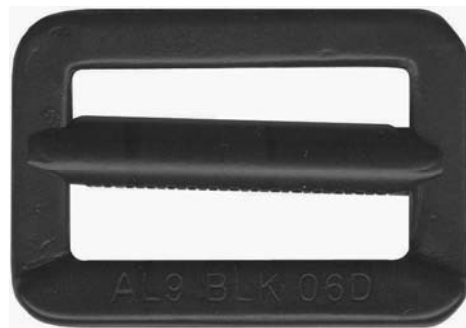
AL9-BLK knurled adjuster bar 1 3/4" x 1" forged steel, black phosphate plated 5,000 lb Commercial version of PS22040
