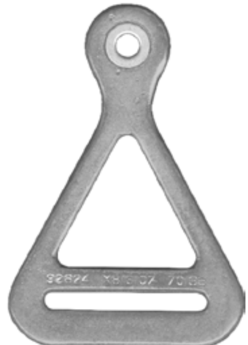
PS173 Bolt-In End Fitting 1 3/4" slot, 1/2" hole steel, cadmium plated Surplus 56B524
