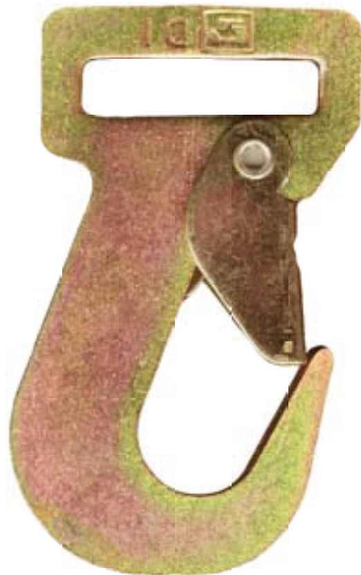
FSN/200-5000 Flat Snap Hook 2" (1 3/4") web slot steel, yellow cadmium plated 5,000 lb.
