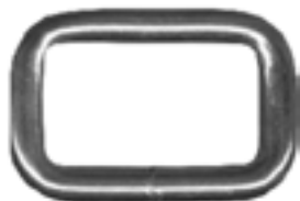
LP3900 Welded Loop 1" x 9/16" .177" steel wire, nickel plated
