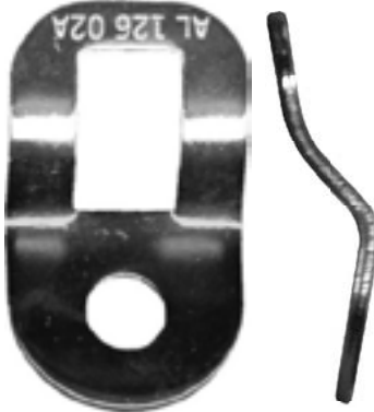
AL126 Bolt-In End Fitting 1/2" slot, 3/8" hole, 45° bend steel, nickel plated 1,000 lb
