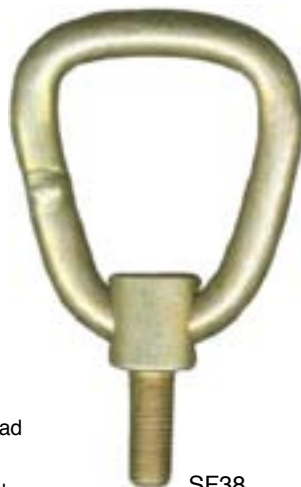
SF38 Stud Fitting - Short Thread with 1" D-Ring steel, yellow cadmium plated 4,000 lb. SPECIAL ORDER
