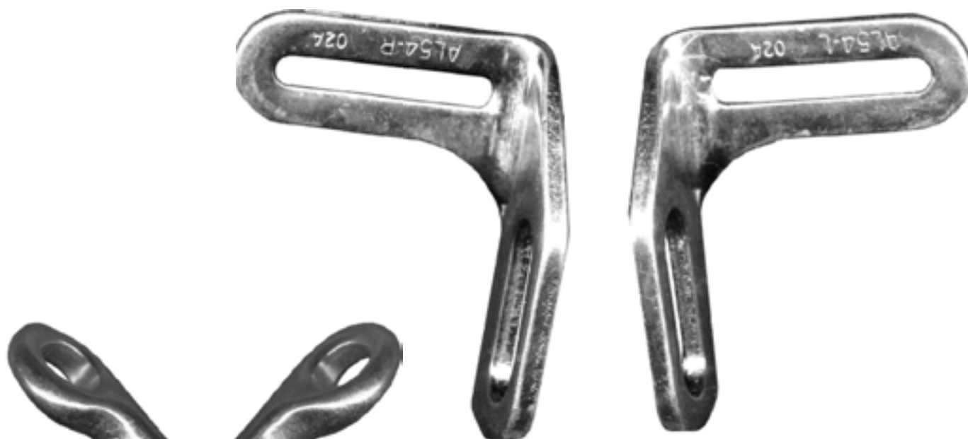
AL54-L & AL54-R Shoulder Links for Latch & Links Left & Right 1 3/4" web slot alloy steel, zinc plated 3,000 lb
