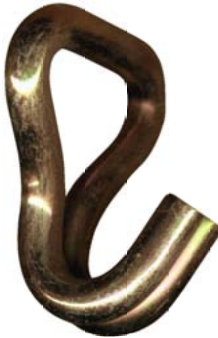
WHK-N/200-10000 Narrow Wire Hook 2" web slot .250" steel wire, yellow cadmium plated 10,000 lb.
