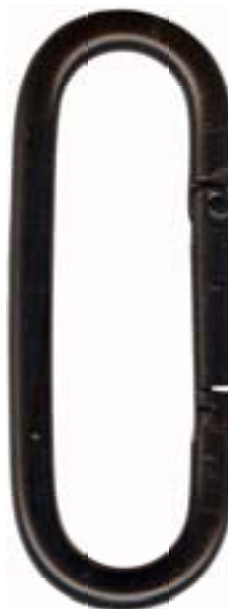
SPO/014-SS 1/4" steel wire, zinc or black resin plated 3 1/8" length 3/8" gate opening SPECIAL ORDER
