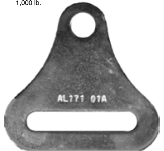
AL171 Bolt-In End Fitting 1 3/4" x 5/16" slot, 3/8" hole alloy steel, nickel plated 3,000 lb
