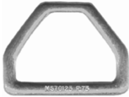
RH39 Accessory D-Ring 1 3/4" forged steel, cadmium plated 1,000 lb. proof load Certifies to PS70123 SPECIAL ORDER
