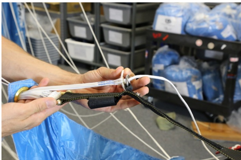
Route Dacron loop through lower brake line cat's eye.
