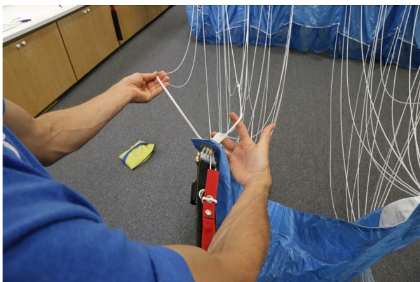
Always ensure correct line continuity after attachment.
