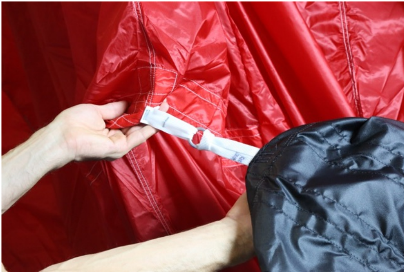
Tighten up lark's head knot
