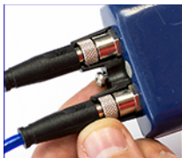
6. Place Connectors Locking Clip (CLC), and check if CLC locks both connectors
