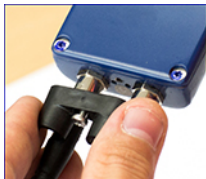
2. Remove Connectors Locking Clip (CLC)
