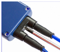
7. After CLC is well positioned, secure with original screw.
