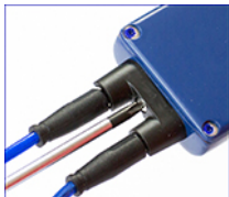
1. Unscrew Connectors Locking Clip (CLC)
