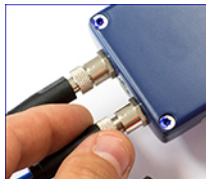
3. Manually unscrew connector of spare unit (for example cutter)
