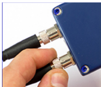
5. Reconnect and manually tighten the new spare unit (Cutter or Control unit)
