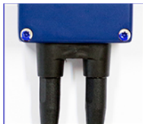
8. Check if CLC is closely attached to Main Box (no space between both objects)
