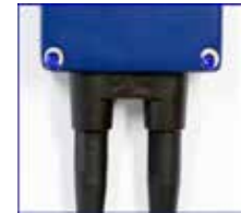
VIII. Check if CLC is closely attached to Main Box (no space between both objects)
