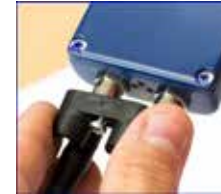
II. Remove Connectors Locking Clip (CLC)
