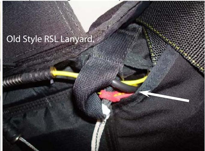
3. The AAD control unit cable must never pass over the RSL lanyard.
