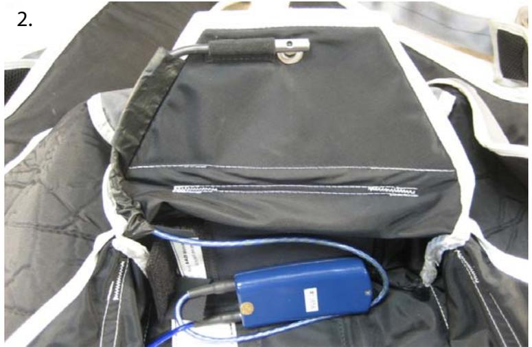
3. Insert the AAD power unit into the spandex pocket as shown.
