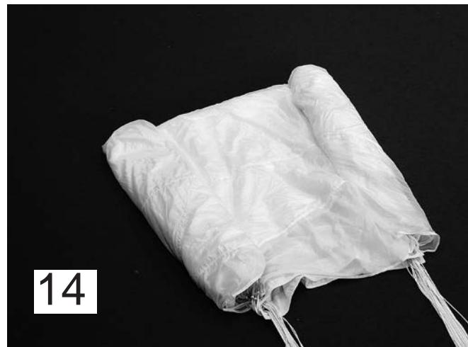
*Slide up the slider and position it carefully in the folds of the center cell, between the two stabilizers.*
