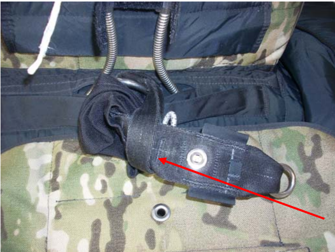
The Drogue Riser separated from the Release Lanyards.
