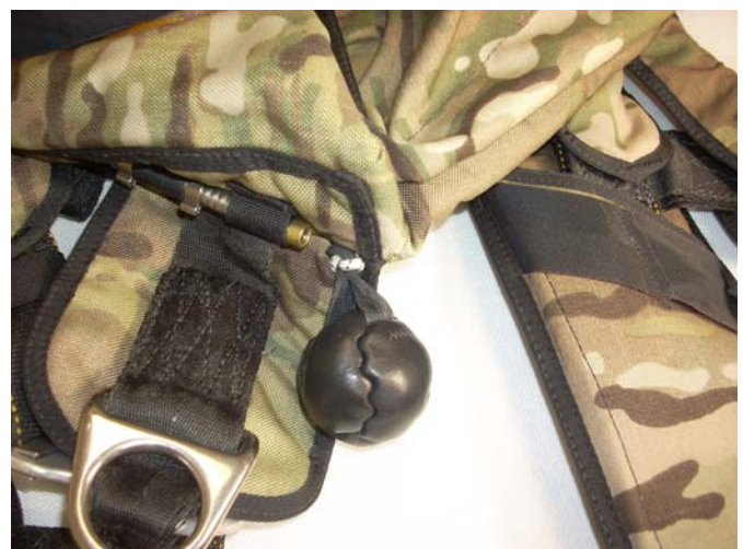
The Lanyard completely removed from the Hacky and the housing.
