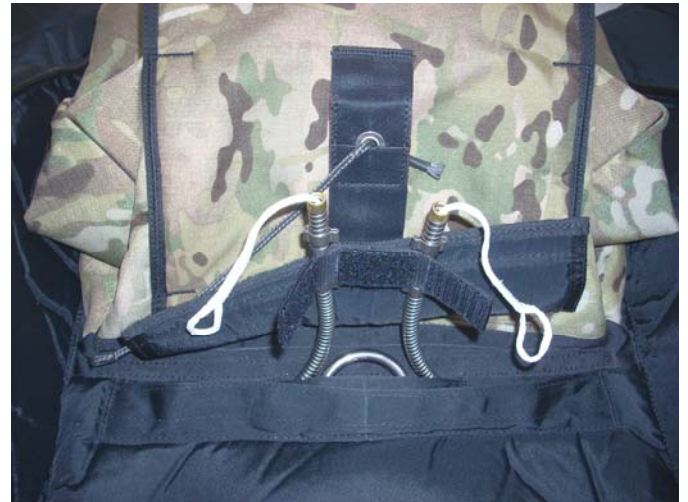
The 3-Ring Drogue Riser removed.
