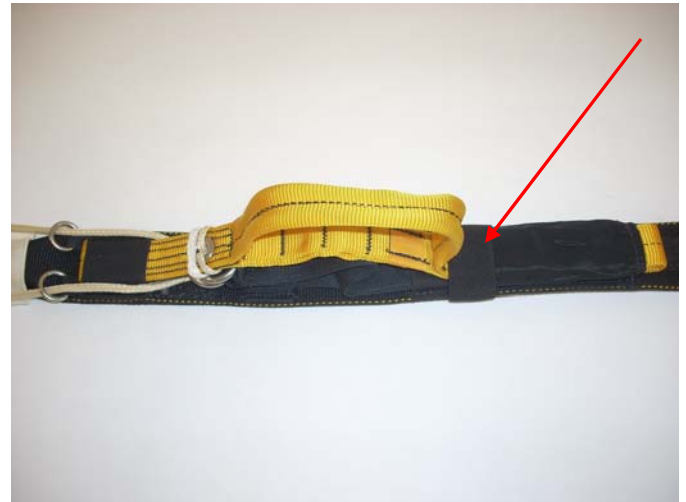
Slide the Elastic Keeper up to the Toggle Loop.
