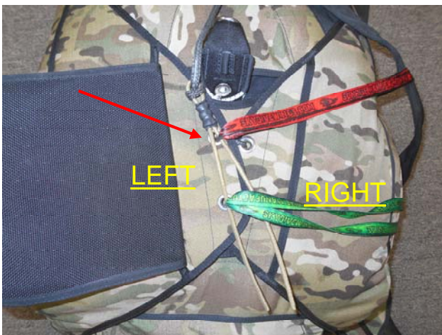
Secure the Safety Closing Loop with the remaining Closing Pin.
