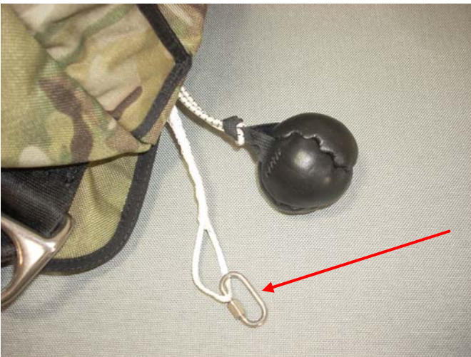
Place the Release Lanyard on a Rapide Link.
