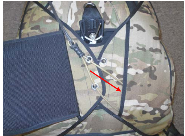
Tuck the ends of the Main Closing Pins into the Right Side Flap .
