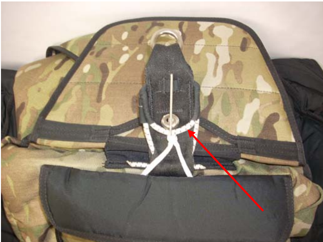
Pictured above is the Drogue Release Pin Elastic (WT-311) on the T-8 Drogue Release Riser.
