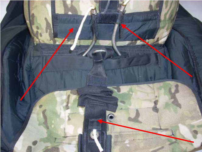
The Drogue Riser separated from the Release Lanyards.
