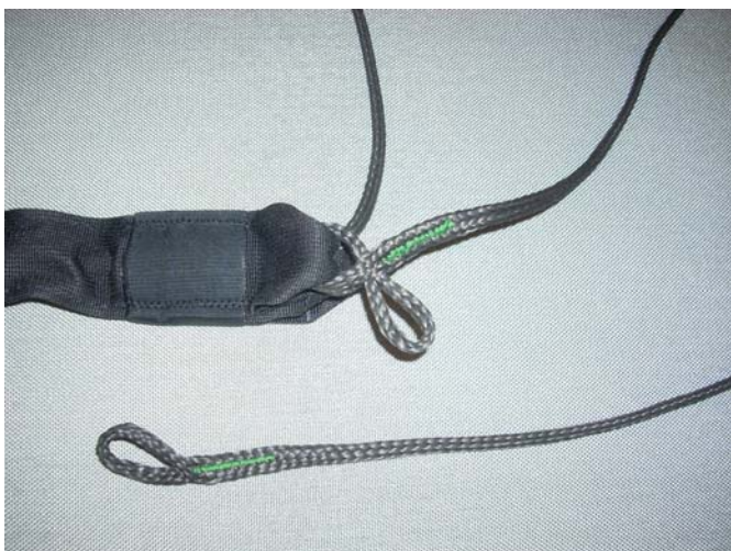
Back the end out through the loop.
