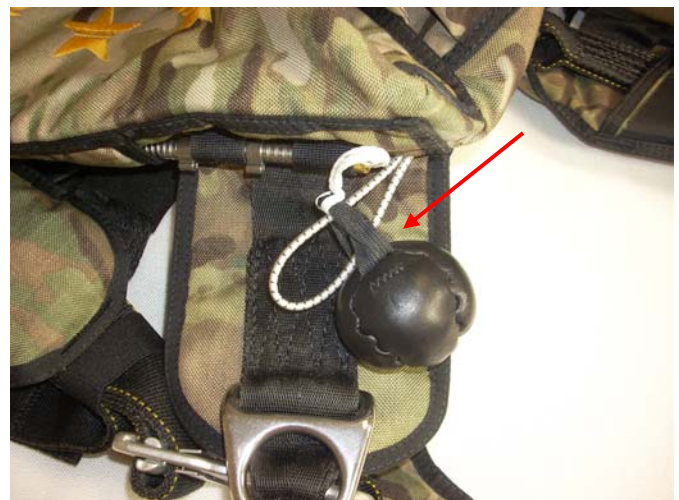
Pass the Connector Loop through the Hacky Handle.
