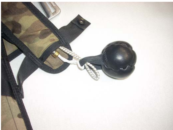
Retractable Connector Loop freed from the Right Release Hacky.
