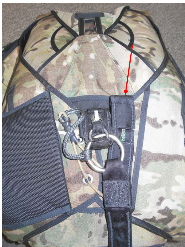
Tuck the Drogue Bridle under the Top Right Side Flap.
