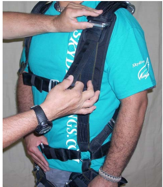
Take out the slack from the main lift webbing.
