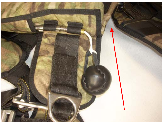
Pull the Connector Loop from the Right Side.
