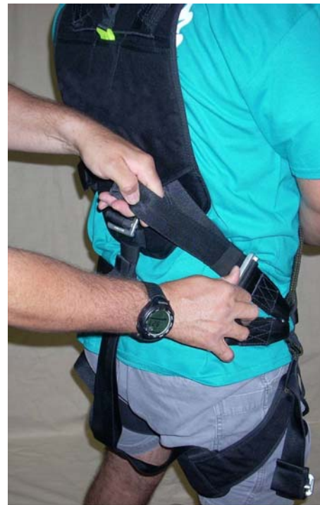
Take out the slack from the back laterals.
