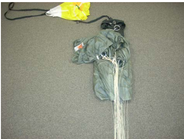
Place the control line group on top of the line groups.
