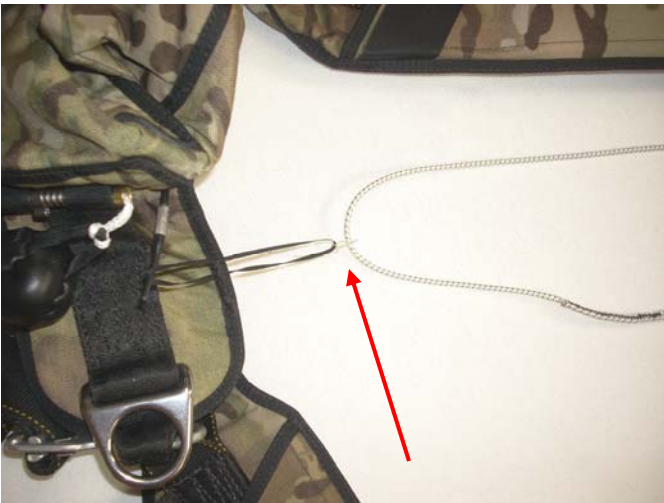
From the left side attach the Retractable Connector Loop to the cleaning rod.
