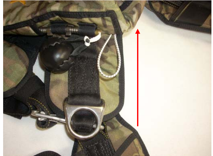
Pull the Connector Loop through the Back Pad from the Right Side leaving 3"-4" out.
