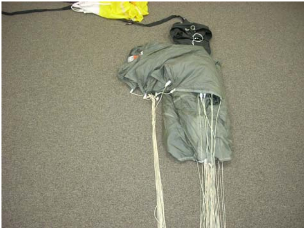
With tension on the C- and D-line groups, fold the D-line section on top of the C-lines.
