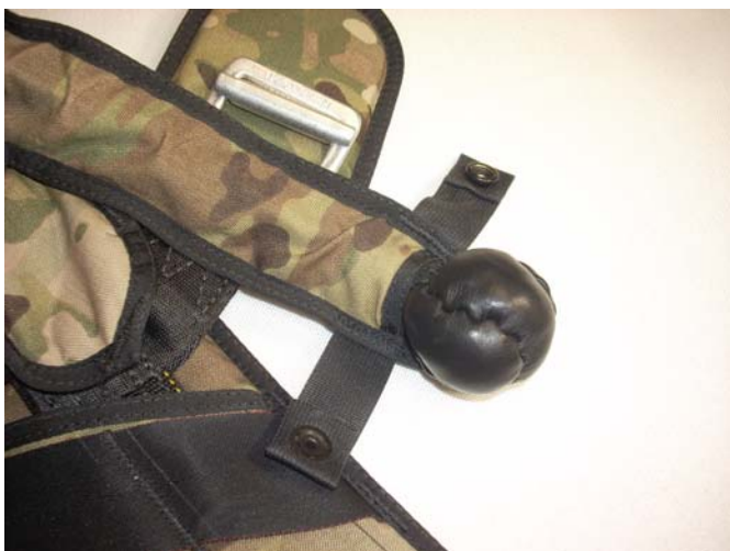
Replacement of the Connector Loop complete.
