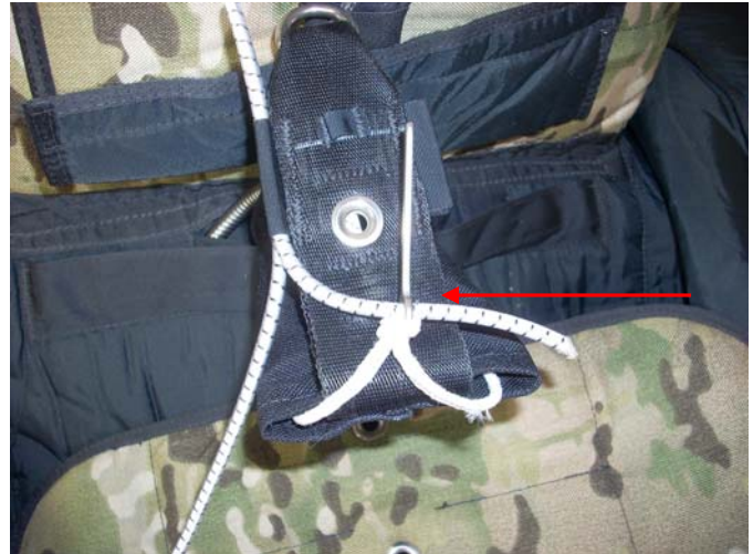
Pass the elastic through the eye of the Straight Pin. (WT-310)
