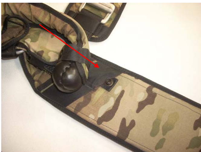
Pass the Snap Holder of the Right Drogue Release Handle under the retainer.
