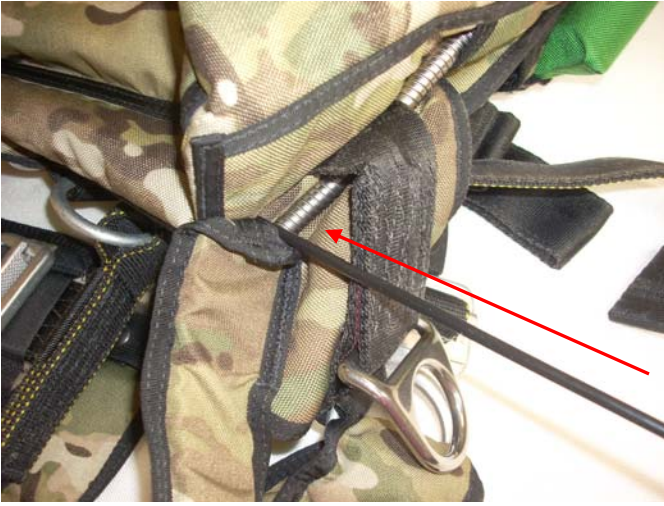
Insert a .22 rifle cleaning rod or similar tool into the opening on the right side of the Handle Sleeve.
