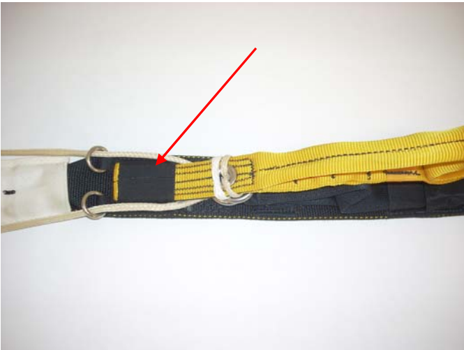
Tuck the Main Steering Toggle into the keeper as shown.
