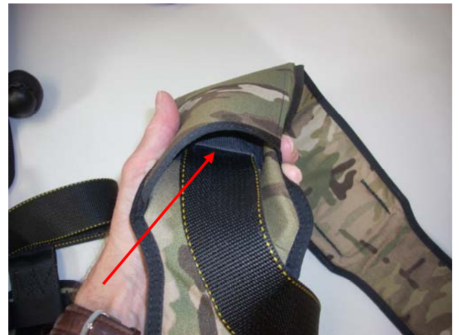
Pass the Leg Strap Webbing under the guide loop.
