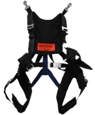
The student harness is secured to the main harness using two 5000-pound butterfly snaps for the upper attachment to the instructor harness, and two 2500-pound adjustable quick ejector snaps for the lower/side attachments. This heavy duty hardware ensures that the student remains secured to the instructor.
