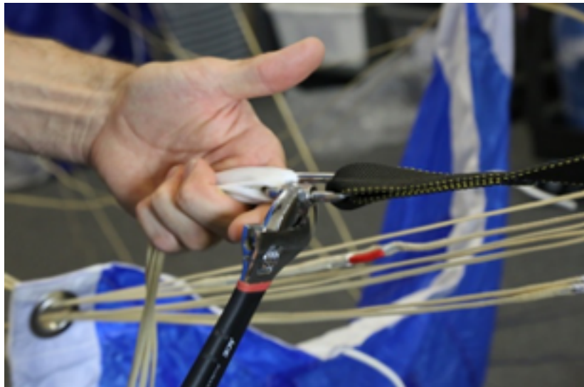
Use a wrench to tighten hard link, approx. 1/8 turn or until appropriately tight. Do not over tighten which may cause damage to link!
