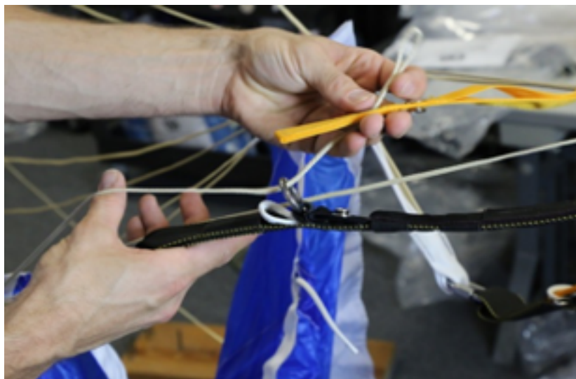
Insert primary control lines through large guide ring, then through primary toggle grommet (gold toggle).
